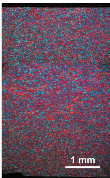
**Figure 5:** AGG is absent after a 65-% deformation and two-stage annealing: 48 h/220 °C + 1 h/480 °C
