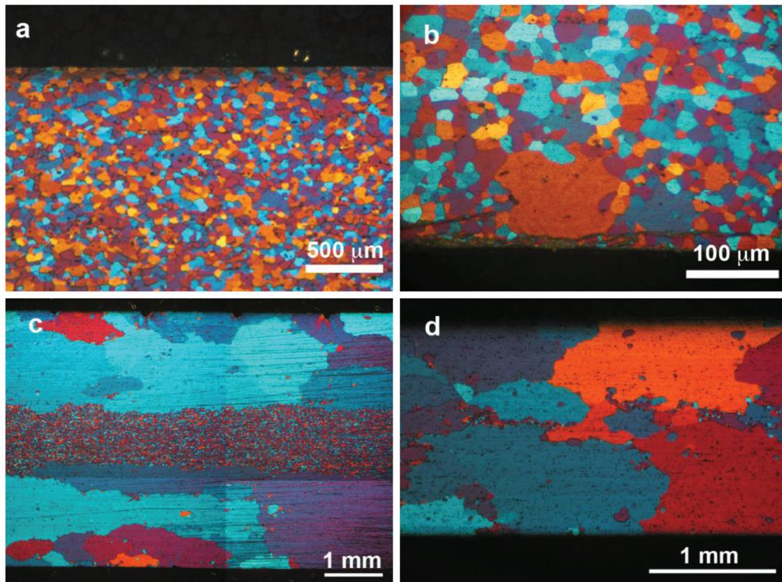
**Figure 4:** Effect of the reduction on the grain growth during annealing at 480 °C for 1 h: (a) 40 %; (b) 50 %; (c) 64 %; (d) 85 %
