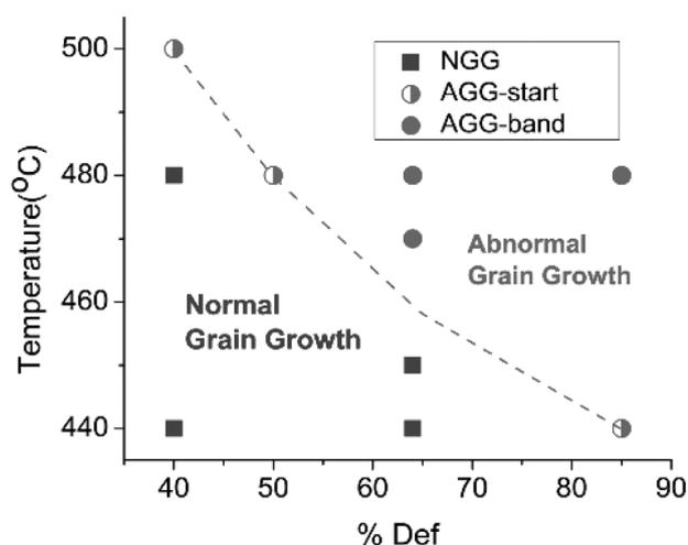
**Figure 6:** Effect of the TMP, degree of reduction and annealing temperature on the grain microstructure and the onset of AGG
