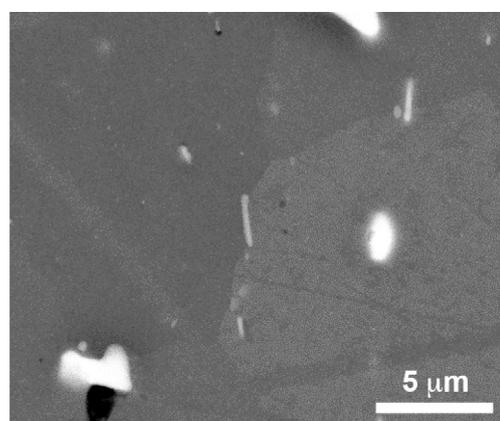
**Figure 3:** Rod-like  $\text{Al}_6\text{Mn}$  particles are more efficient at pinning grain boundaries in the RD due to the longer axis aligned parallel to the RD (5 min/480 °C)
