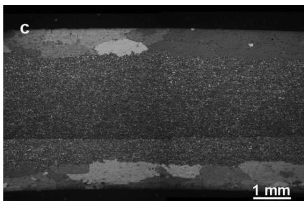
**Figure 2:** Effect of the annealing time on AGG during annealing at 480 °C: a) 5 min, b) size (eq. diameter) vs shape (roundness) of abnormal grains after 5-min annealing, c) 15-min annealing
