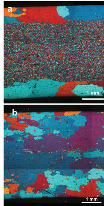
**Figure 1:** Effect of the temperature on AGG during isochronal annealing (1h): a) 470 °C, b) 520 °C
