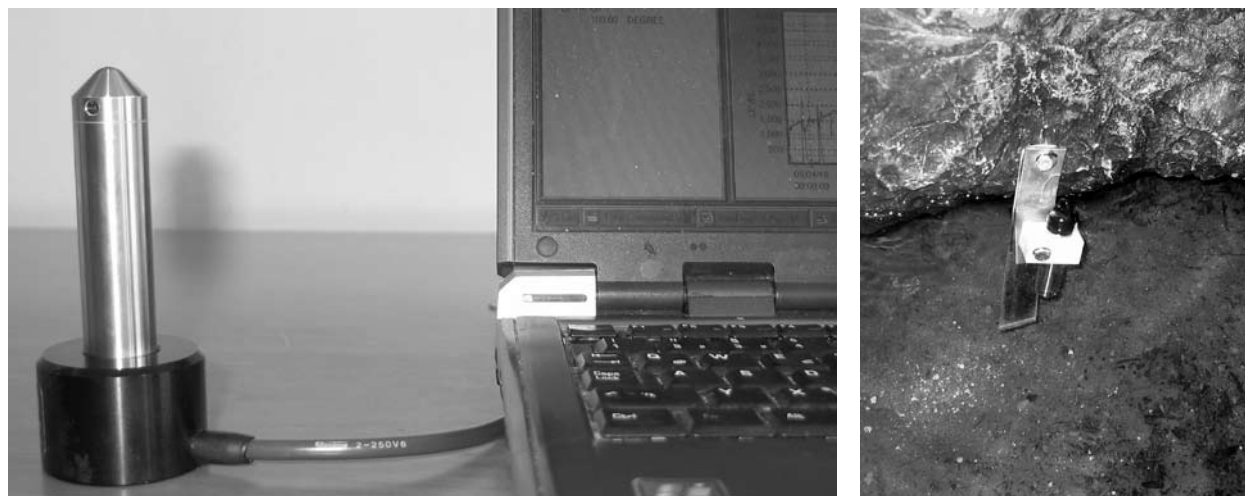
Fig. 3: Datalogger in the office, connected to the computer via optical reader (left) and fixed to the wall of the terminate lake of Jama 1 v Kanjeducah (P3) (right).
