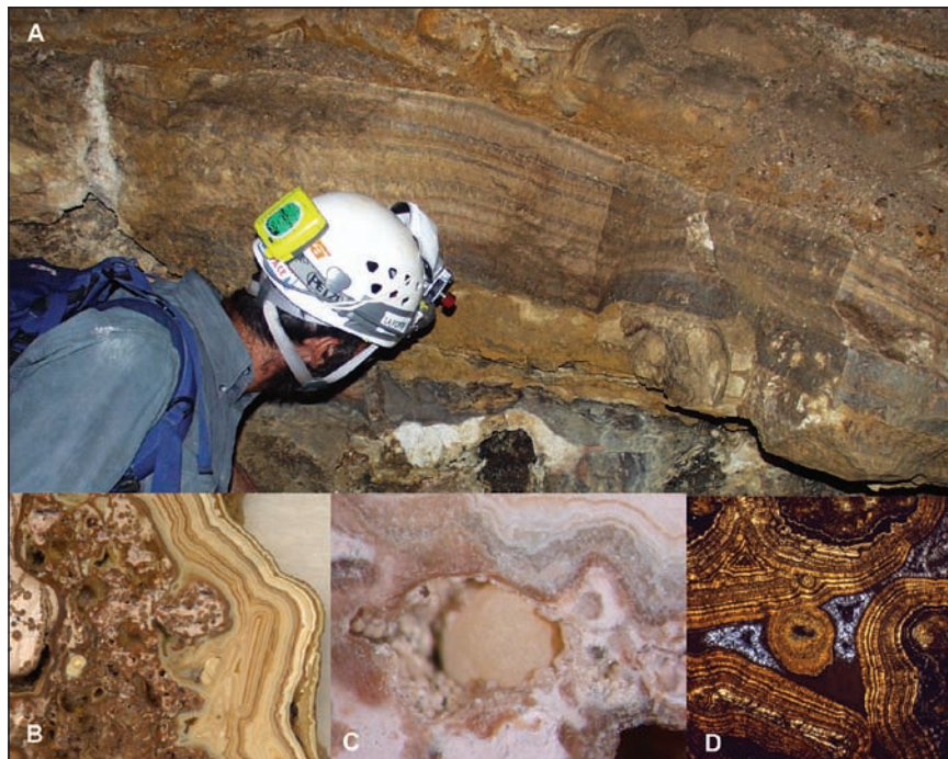
Fig. 12: Cueva Rossillo: a) a thick phosphate flowstone developed in the final part of the cave; b) layers different in colour and/or texture are evident in a polished cross section; c) microsphere of pale yellow ardealite in a small void of the speleothem; d) the different layers observed with a polarizing microscope with crossed nicols.
