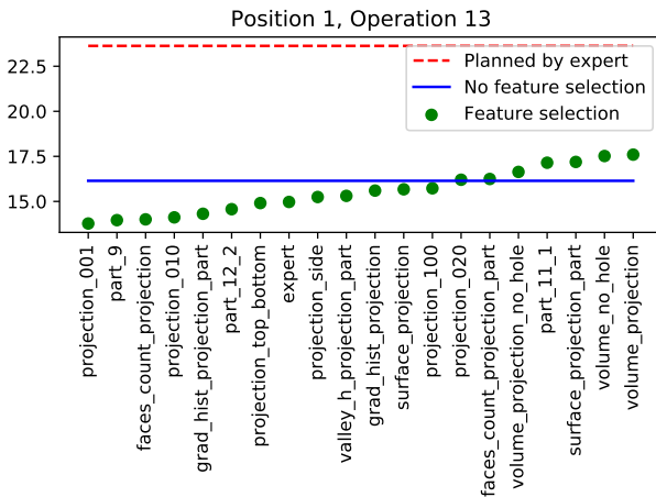
Figure 4: RMSE obtained when predicting the duration of operation 13 (submersible erosion) at position 1.
