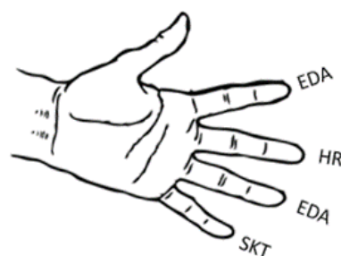
Figure 1: Illustrated human hand with corresponding signals measured on finger pads. Electrodermal activity on the index and ring finger, heart rate on the middle finger, and skin temperature on the little finger
