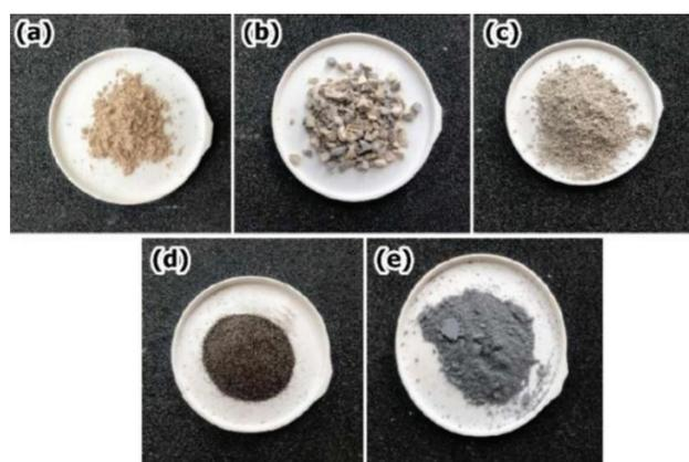
**Figure 2:** Raw materials: a) RC, b) CC, c) FC, d) GGWS, and e) AC
