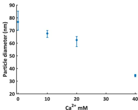
Figure 4: Decrease in liposome particle diameter with respect to concentration of calcium solution added to the liposome sample. The error bars represent the cutoff frequency of the obtained distribution.
