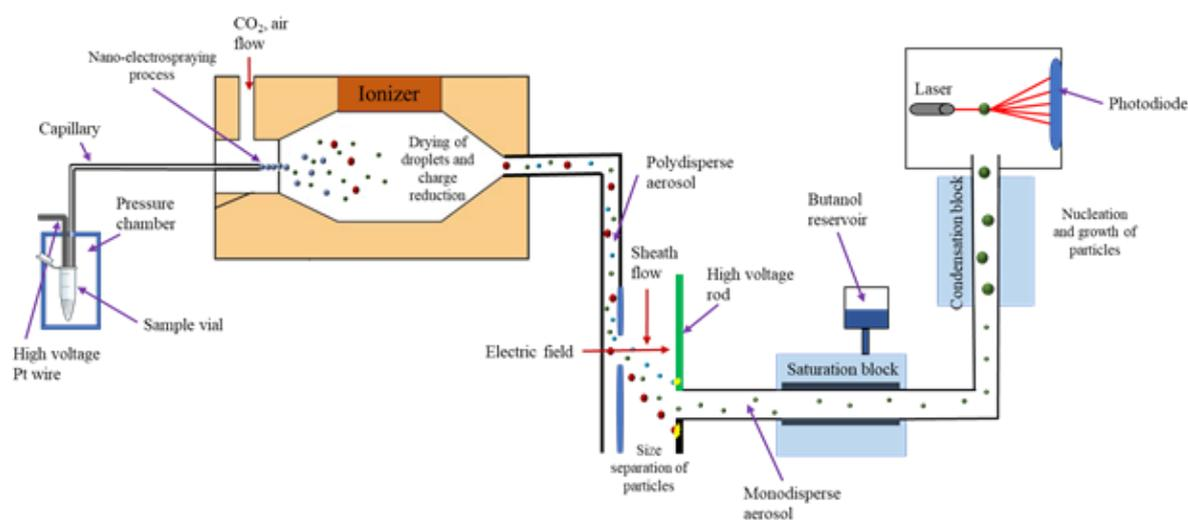
Figure 2: Schematic presentation of nES GEMMA working principle. The first part consists of a nano electro spray based aerosol generator where aerosol is generated from our sample. Polydisperse aerosol then flows through the nano-differential mobility analyser where the particles get classified based on their size. In the end, monodisperse particles are detected by a condensation particle counter.
