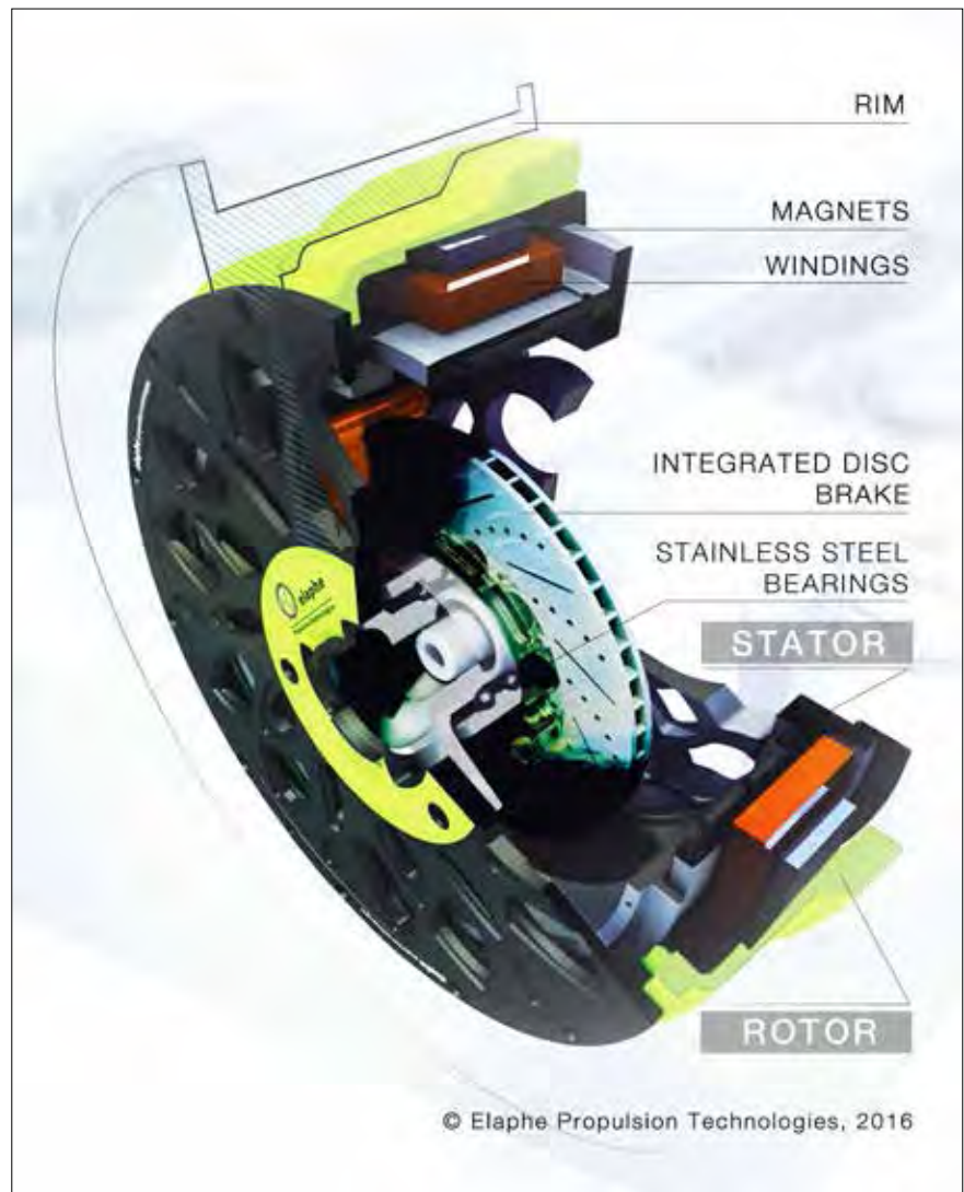
Figure 2. Elaphe M700 in-wheel motor cross-section. The motor fits inside a regular 16" or larger rim and is integrated with standard off-the-shelf parts like the hub bearing and friction brake. Windings are part of the inner stator and the magnets are attached to the inside of the outer rotor shell.
