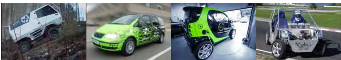
Figure 5. A selection of vehicles using Elaphe electric motors as the propulsion system of choice. (1 -Steinbock HX1 all-terrain vehicle with 4 in-wheel motors, 2 – VW Sharan through-the-road hybrid, with 2 near-wheel motors, 3 - Smart pure-electric car with 2 in-wheel motors in the rear, 4 – Chebela, a pure electric Slovenian concept car with 2 in-wheel motors.
