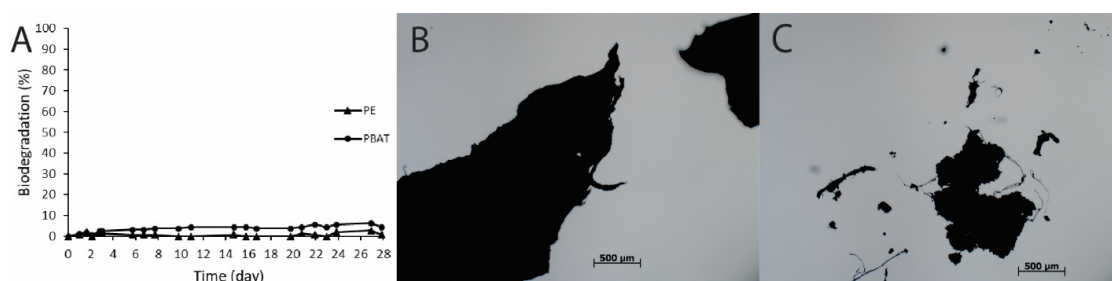
Figure 1: A) Biodegradation of PE and PBAT, B) Optical microscopy image of PBAT, C) Optical microscopy image of PE.
