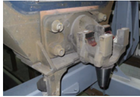
Figure 3: Flange with conical stud
