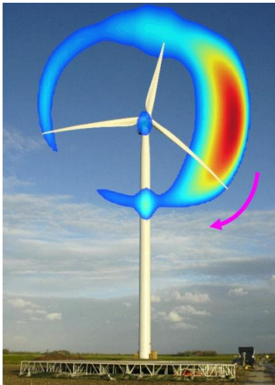
Figure 3. Location and quantification of noise sources on a wind turbine (Oerlemans et al., 2007).
