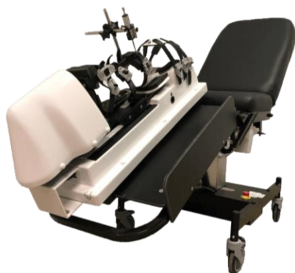
Figure 1. The DYNEELAX® arthrometer set up to measure the laxity of the right knee joint (Genourob, n.d.).
