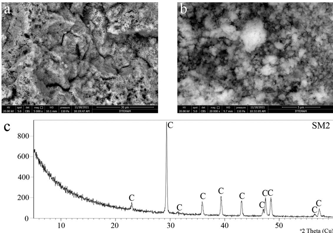
**Figure 2:** Typical lime lump (SM2 sample) consisting of micritic calcite crystals: a) SEM 5000 $\times$ , b) SEM 20000 $\times$ , c) XRD pattern (C: calcite 86-2334)
