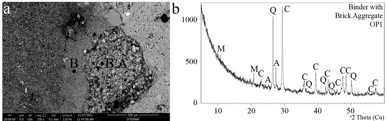
**Figure 5:** Binder (B) with a brick aggregate (B.A.) – sample OPI: a) SEM image 250x, b) XRD pattern (A: albite 76–1819, C: calcite 86–2334, M: muscovite 84–1302, Q: quartz 85–0798)
