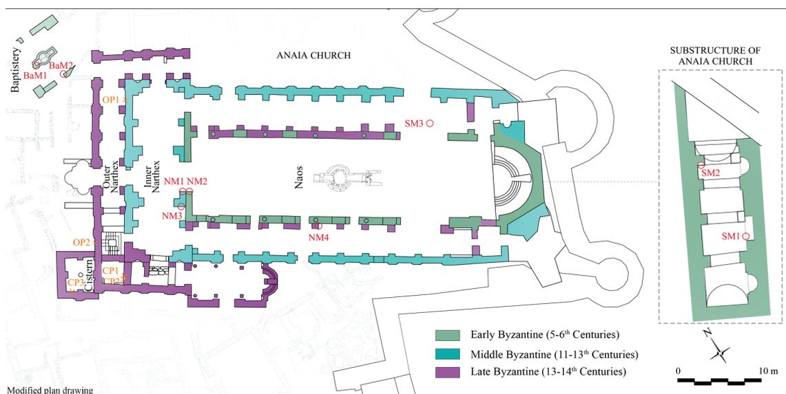
**Figure 1:** Plan showing the construction periods of the Anaia Church and sample locations
