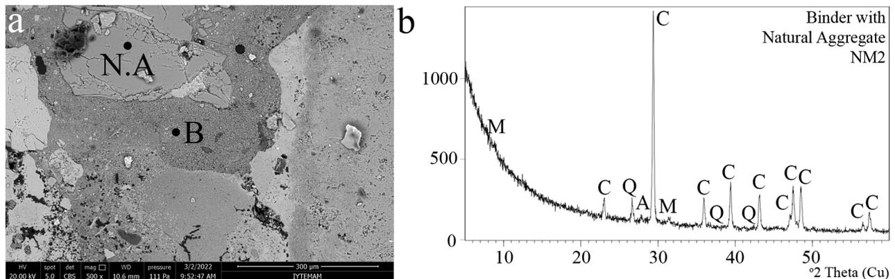
**Figure 6:** Binder (B) with a natural aggregate (N.A.) – sample NM2: a) SEM image 500x, b) XRD pattern (A: albite 76–1819, C: calcite 86–2334, M: muscovite 84–1302, Q: quartz 85–0798)
