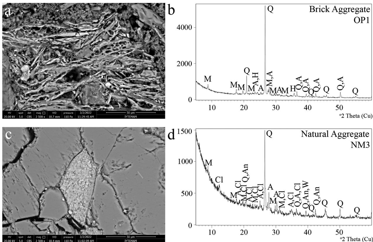
**Figure 4:** SEM images and XRD diffraction patterns of the aggregates: a) brick SEM 2500x, b) brick XRD, c) natural SEM 2500x, d) natural XRD (A: albite 76–1819, Cl: clinocllore 79–1270, H: hematite 87–1166, M: muscovite 84–1302, Q: quartz 85–0798)
