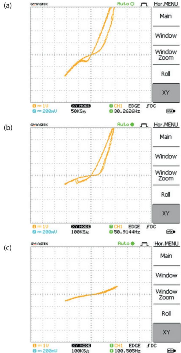
**Figure 6:** The hysteresis curve of the Tungsten-based memristor fed with a a) 30, b) 50 Hz, and c) 100 Hz and a 2 V peak-to-peak sinusoidal voltage.
