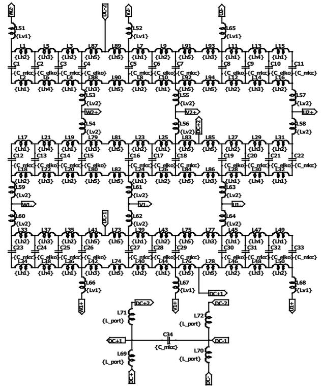
Figure 6: LTspice® model of the DC link.
