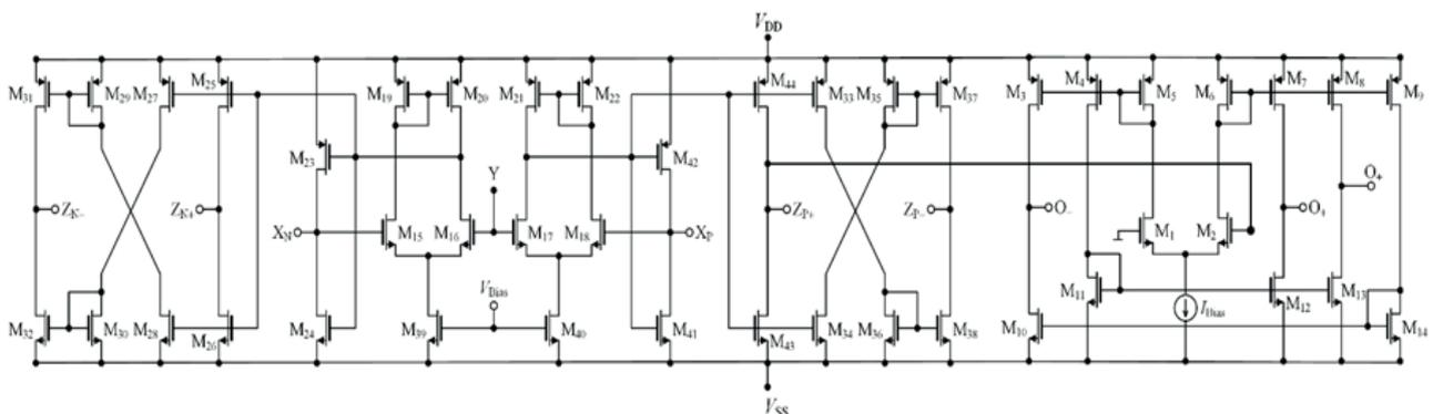
Figure 3: The CMOS implementation of EXCCTA
