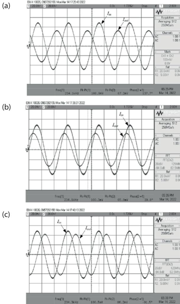
**Figure 25:** Time domain Analysis of CM configuration: (a) LP (b) HP (c) AP
