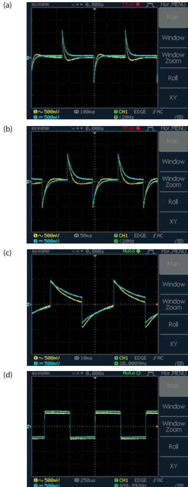
**Figure 10:** The current of the Tungsten-based memristor and the voltage waveform at node D2 when the M-C-R<sub>s</sub> series circuit is fed with a a) 2 Hz, b) 5 Hz, c) 20 Hz, and d) 1 kHz, and a 2 V peak-to-peak square wave voltage.
