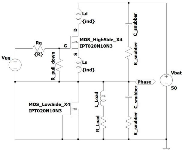
Figure 9: Test configuration featuring the clamped inductive load with  $V_{gg}$  controlling the high side MOS-FETs. The measurements were taken using an inductive load of  $40 \mu\text{H}$  and  $6.66 \Omega$ , achieving a current of  $400 \text{ A}_{\text{DC}}$  with the correct duty cycle, the  $V_{\text{DC}}$  was  $50 \text{ V}$ .
