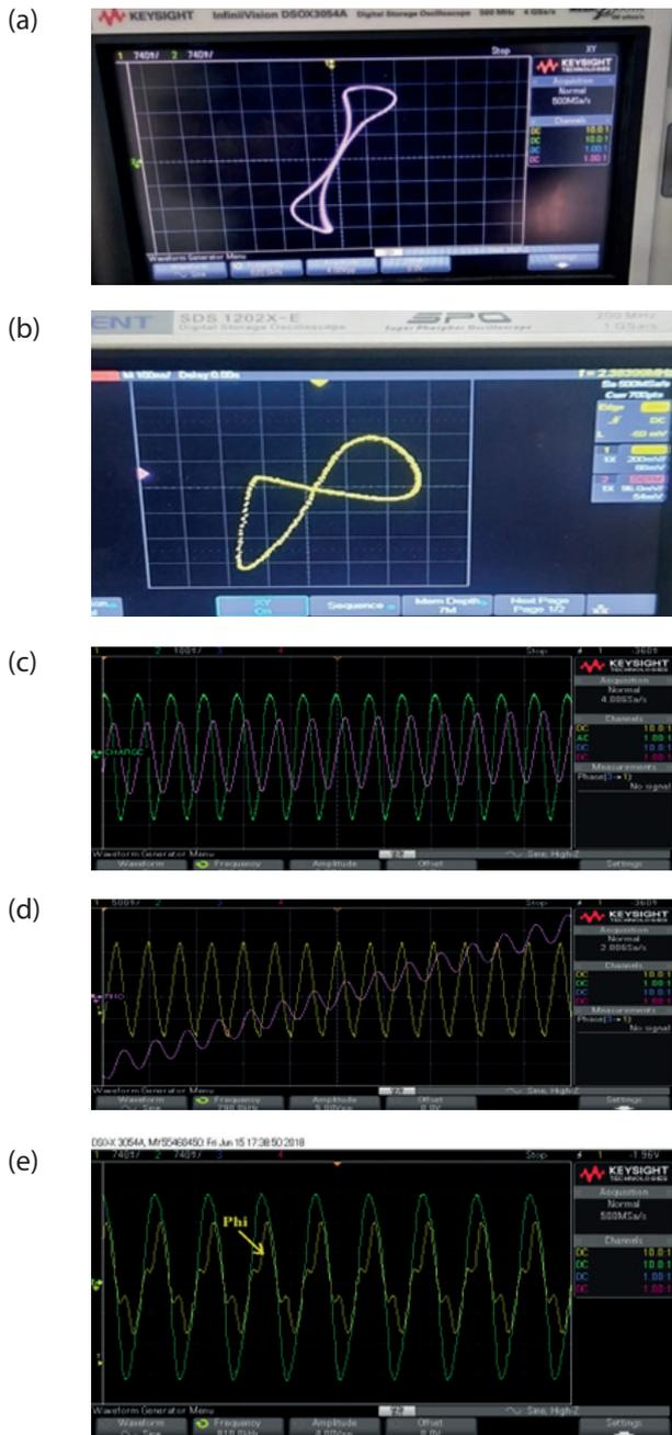
**Figure 22:** Experimental Results of meminductor emulator (a) hysteresis loop for grounded meminductor, (b) hysteresis loop for floating meminductor, (c) time domain waveform for Current (Green) and Charge (pink), (d) time domain waveform for phi (yellow) and rho (pink), (e) time domain waveform for phi (nonlinear) and current (sinusoidal).
