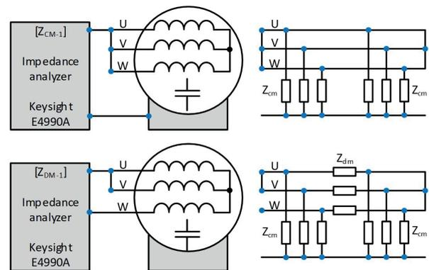
Figure 11: Common mode test configuration with motor equivalent impedance  $Z_{\text{CM-1}}$  and differential mode test configuration with  $Z_{\text{DM-1}}$  [13].
