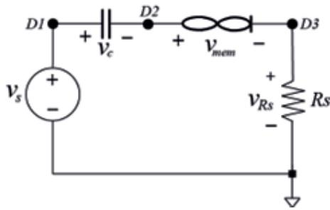
**Figure 9:** The Tungsten-based memristor-capacitor-protection resistor (M-C-R<sub>s</sub>) series circuit excited with a square wave voltage source.
