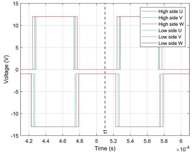
Figure 19: Static PWM1 switching sequence at  $t_1$ .
