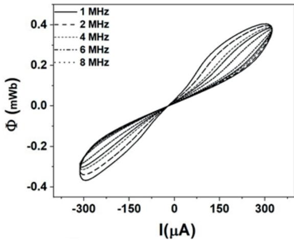
**Figure 8:**  $\Phi$ -I characteristic for floating meminductor circuit at different operating frequencies for  $A_m = 200$  mV,  $I_{b2} = 20$   $\mu$ A,  $V_{B4} = 0.5$  V,  $C_1 = 150$  pF,  $R = 5$   $\Omega$  and constant  $C_2 f = 75 \times 10^{-6}$  FaradHz.
