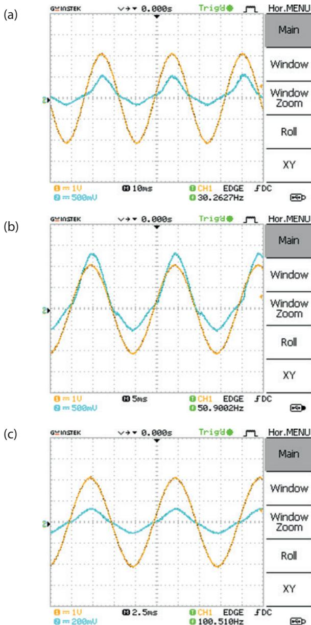
**Figure 5:** The time-dependent current and voltage waveforms of the Tungsten-based memristor fed with a a) 30, b) 50 Hz, and c) 100 Hz and a 2 V peak-to-peak sinusoidal voltage.
