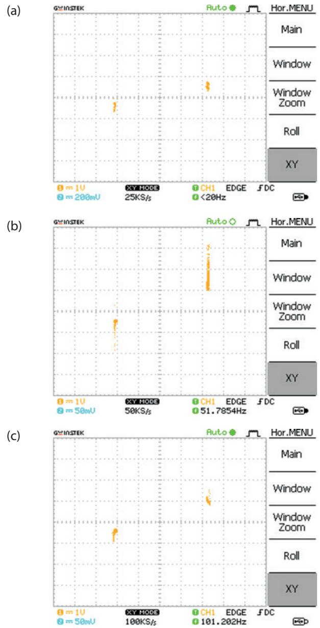
**Figure 8:** The hysteresis curve of the Tungsten-based memristor fed with a) 20 Hz, b) 50 Hz, c) 100 Hz, and an approximately 2.4 V peak-to-peak square voltage.
