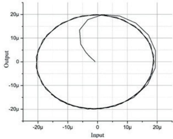
**Figure 8:** Lissajous patterns for CM AP configuration
