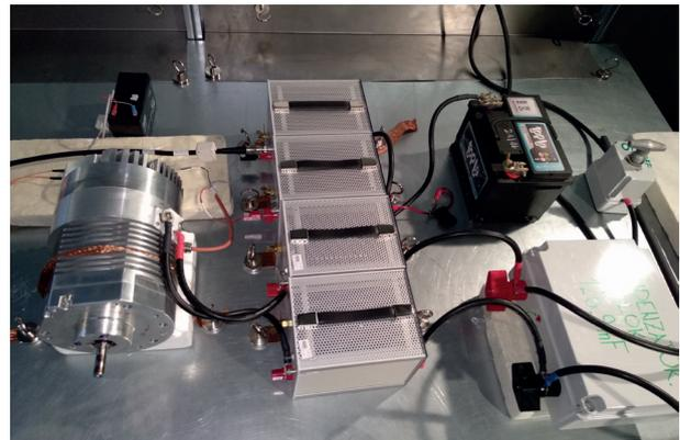
**Figure 1:** MAHLE 48 V 11.2 kW integrated motor drive with test setup according to CISPR 25.
