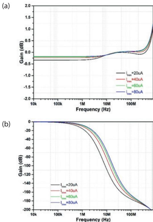
**Figure 7:** Tunability of CM AP response for different values of bias currents: (a) Gain (b) Phase
