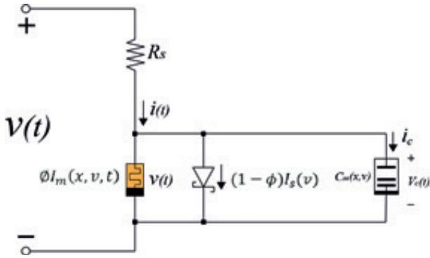
**Figure 15:** The equivalent circuit of the Tungsten-based Known Memristor.
