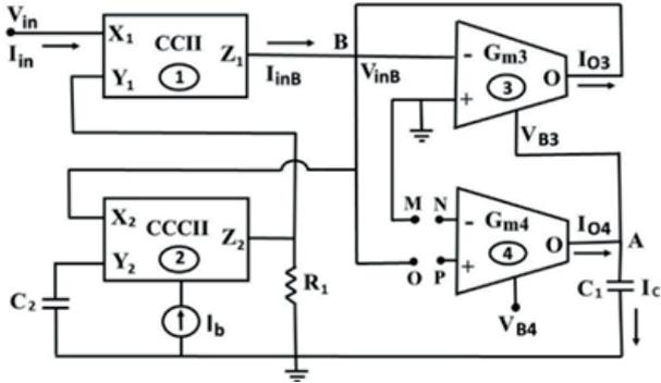
**Figure 4:** Schematic diagram of grounded meminductor emulator.
