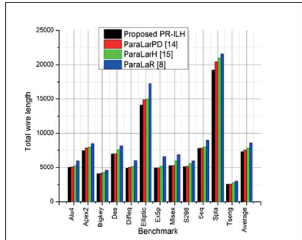
**Figure 3:** Comparison of total wire length for the proposed PR-ILH, ParaLarPD [14], ParaLarH [15], and ParaLaR [8].
