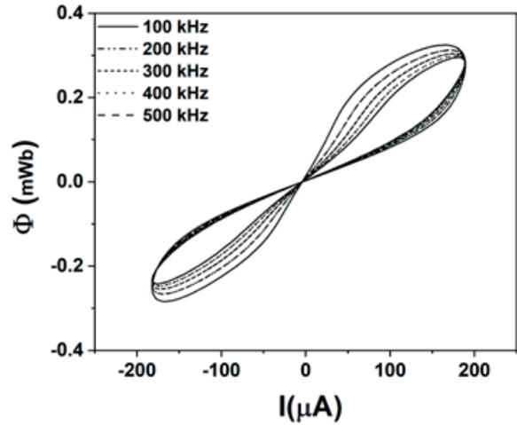
**Figure 6:**  $\Phi$ -I characteristic for grounded meminductor circuit at different operating frequencies for  $A_m = 140$  mV,  $I_b=20 \mu$ A,  $V_{B4} = 0.45$  V,  $C_1 = 150$  pF,  $R=10 \Omega$  and constant  $C_2f=75 \times 10^{-6}$  FaradHz.
