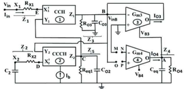
Figure 17: Non-ideal model of grounded meminductor emulator.
