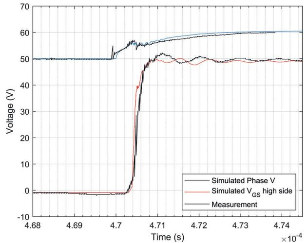
Figure 10: Switching sequence – high side ON.  $V_{\text{GS}}$  has an offset of  $+50 \text{ V}$  for figure clarity.
