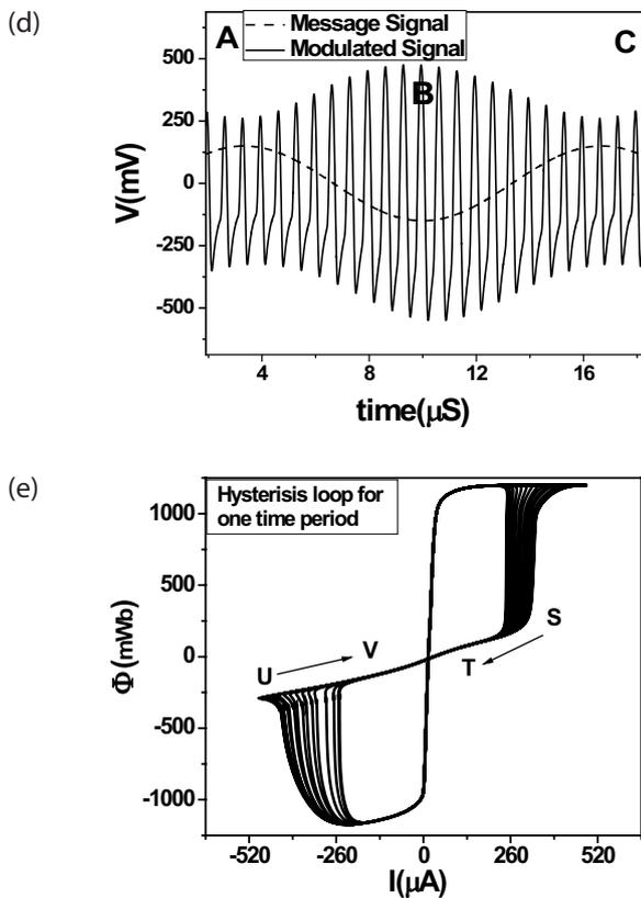
**Figure 20:** The plot of (a) carrier signal, message signal, and modulated signal, (b) spectrum of the modulated signal, (c) recovered message signal, (d) waveform of message and carrier for one period, (e) hysteresis loop of AM for one period.
