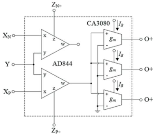
**Figure 22:** Implementation of EXCCTA using off the shelf ICs
