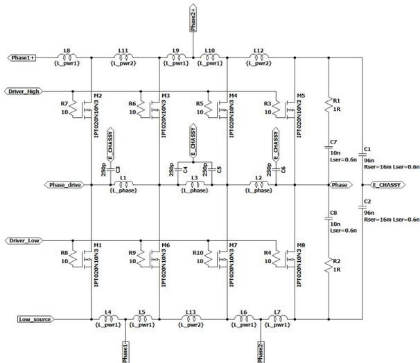
Figure 8: Power board single phase LTspice® model.
