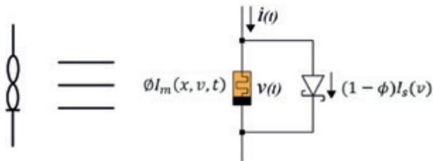
**Figure 2:** The equivalent circuit of a Tungsten-based Knowm memristor [43].
