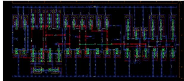
Figure 4: The layout of EXCCTA in 180nm technology
