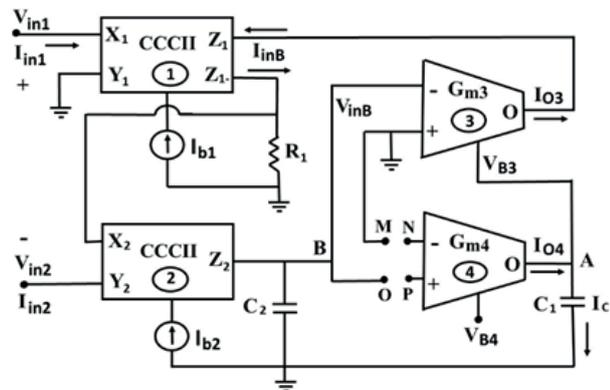
**Figure 5:** Schematic diagram of floating meminductor emulator.
