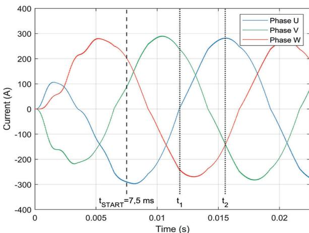
Figure 18: Simulated phase currents based on the SVPWM control strategy ( $t_{START}$  is the starting time for post-processing,  $t_1$  and  $t_2$  are times of the arbitrarily chosen static PWM switching sequences).
