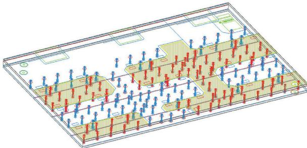
Figure 5: DC link PCB (Ansys® Slwave™).
