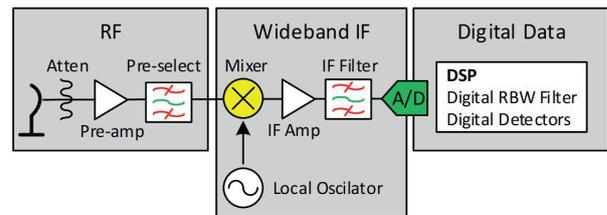
**Figure 14:** Block diagram of the FFT based EMI receiver [20].
