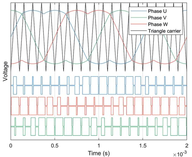
**Figure 24:** SVPWM control strategy (the chosen sequence is for figure clarity only and does not match the operating point at 1000 RPM).
