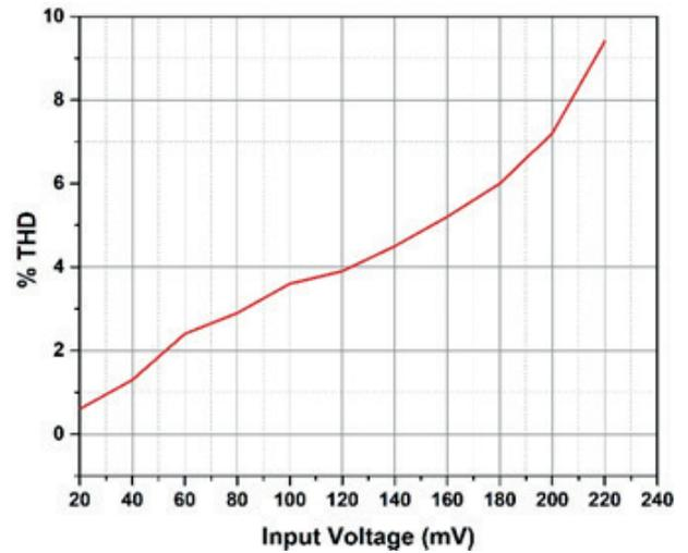
**Figure 18:** Total harmonic distortion of VM AP configuration
