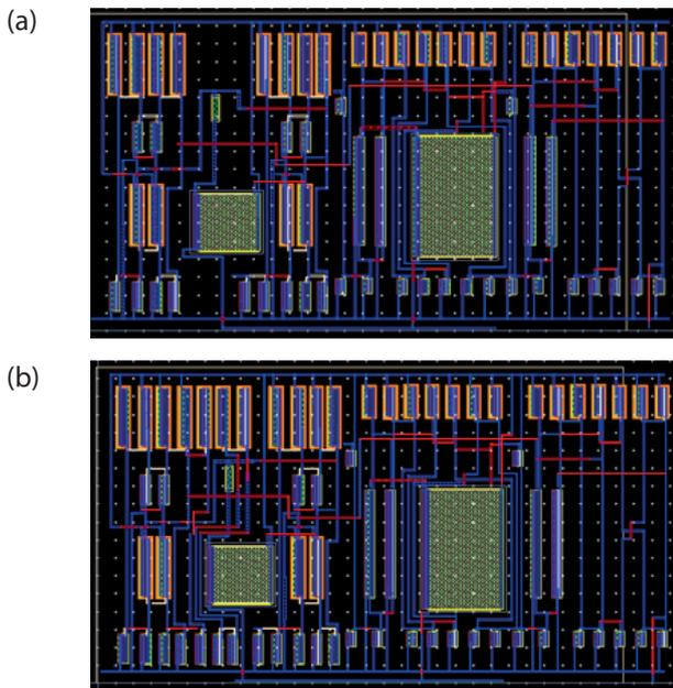
**Figure 12:** Layout of meminductor emulators (a) grounded (b) floating.
