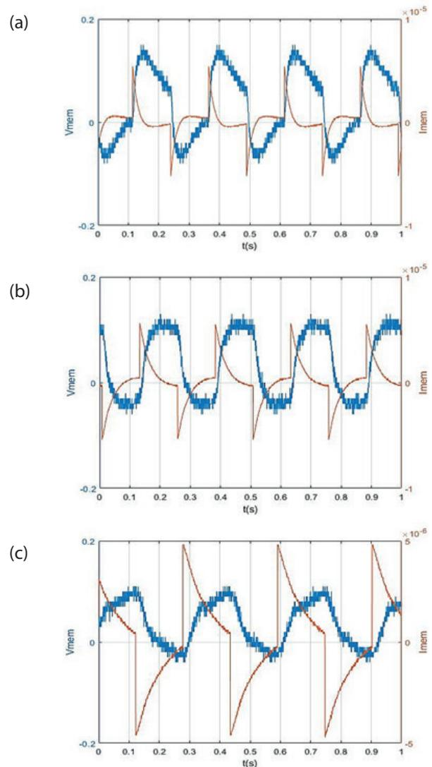
**Figure 11:** The time-dependent current and voltage waveforms of the Tungsten-based memristor when the M-C-R<sub>s</sub> series circuit is fed with a a) 5 Hz, b) 10 Hz, and c) 20 Hz, and a 2 V peak-to-peak square wave voltage.
