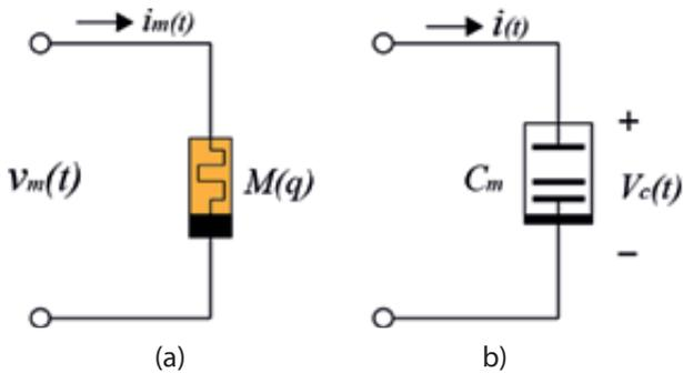
**Figure 1:** a) Memristor and b) Memcapacitor symbols.
