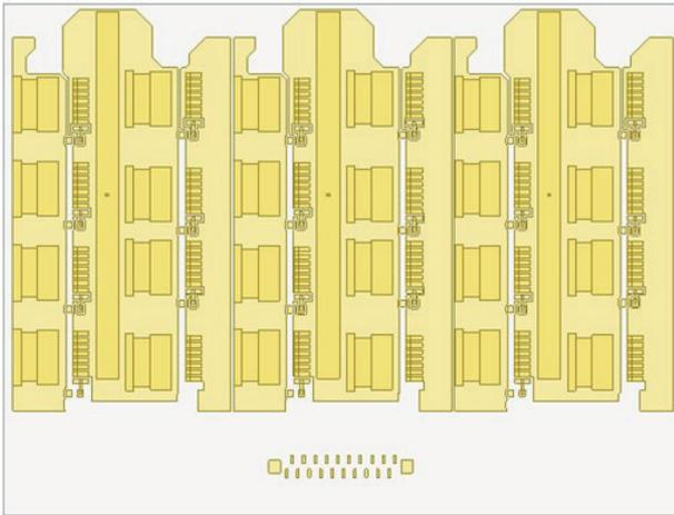
Figure 7: Power board PCB planes (Ansys® Slwave™).
