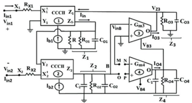
**Figure 18:** Non-Ideal model of proposed floating meminductor emulator.
