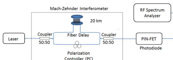
Figure 1. Delayed self-homodyne technique
