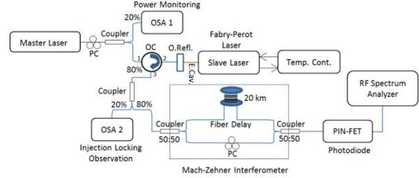
Figure 7. Experimental set-up for injection locking and linewidth observation using the delayed self-homodyne technique.
