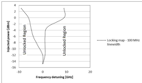
Figure 6. Injection locking map of the FP laser
