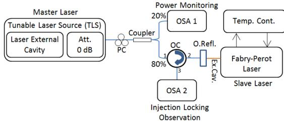
Figure 4. Experimental set-up for injection locking
