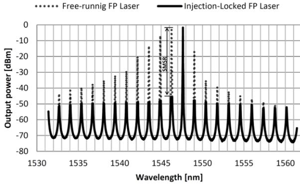
Figure 5. Optical spectrum of the FP laser
