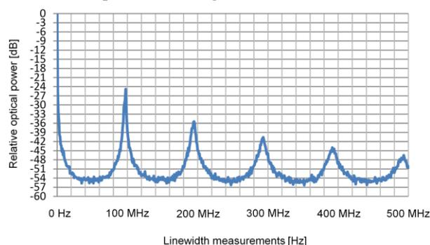
Figure 3. Linewidth measurements for the multi-longitudinal-mode laser
