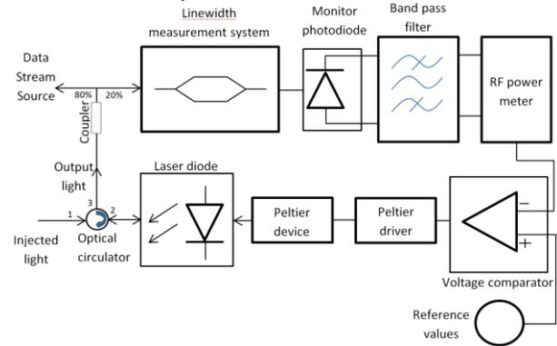
Figure 9. Self-restorable architecture for stable injection locking of a FP laser
