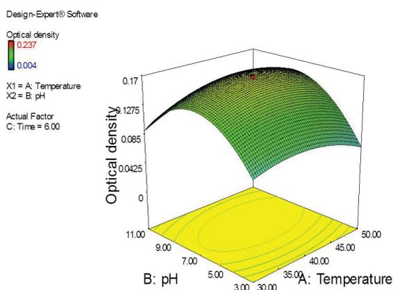
**Figure 1:** Surface and contour plot showing effect of temperature and pH on bitumen degradation (optical density).
