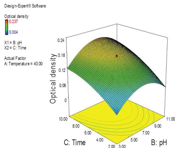
**Figure 3:** Surface and contour plot showing the effect of pH and time on bitumen degradation (optical density).
