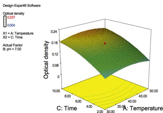
**Figure 2:** Surface and contour plot showing the effect of temperature and time on bitumen degradation (optical density).
