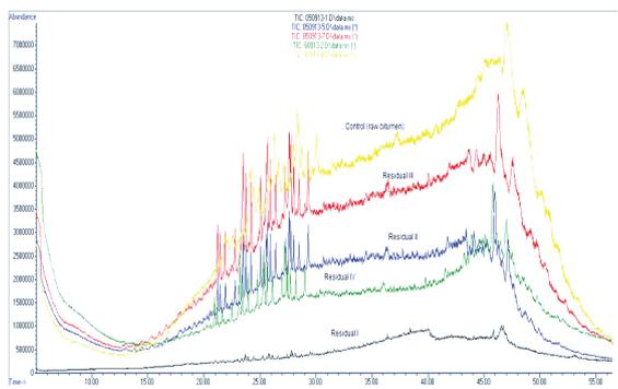
**Figure 4:** The Total Ion Chromatogram (TIC) of the control sample and the extracts of the residual degraded bitumen.
