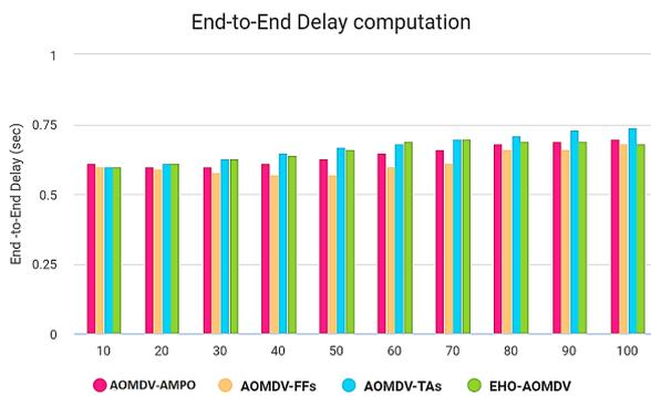
**Figure 14:** Computation of latency vs faulty nodes
