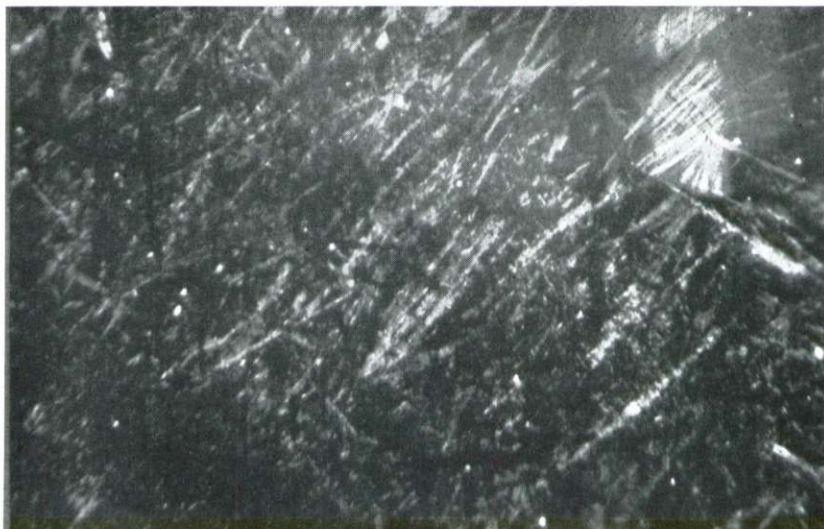
Pl. IV., Fig. 1. Ghedem ore; — oil immersion, crossed nicols, 135 \times . Fine-crystalline aggregate of pyrolusite
