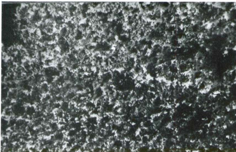
Pl. III., Fig. 1. Mai Gudo ore; — oil immersion, 135 \times . Porous impure limonitic ore
