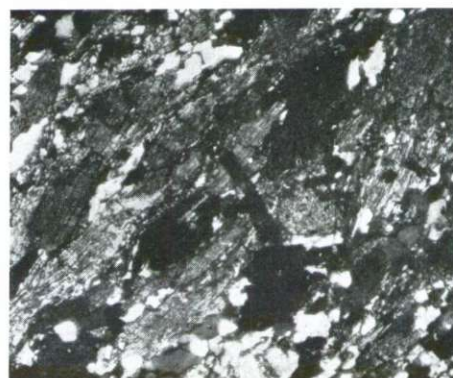
Fig. 3. Amphibolite (grains of hornblende in groundmass of salic minerals) \times 35 . Gayo Camp. Determination A. Hinterlechner
