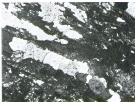
Fig. 1. Zoisite-amphibole schist (quartz, zoisite, hornblende, epidote), \times 35 . Bedakessa, Adola district. Determination A. Hinterlechner
