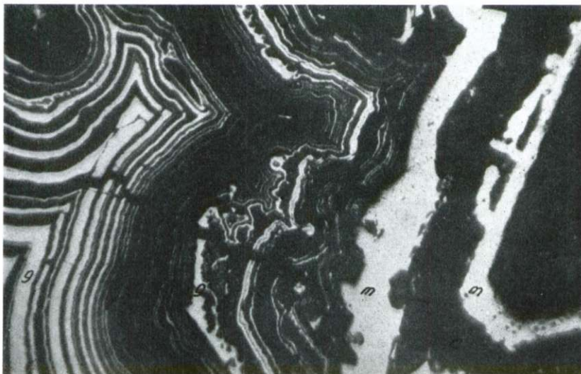
Pl. III., Fig. 2. Ghedem ore; — oil immersion, 135 \times . Zonal texture of ore, consisting of alternating bands of iron oxide (g), manganese oxide (m), silica (s) and calcite (c)
