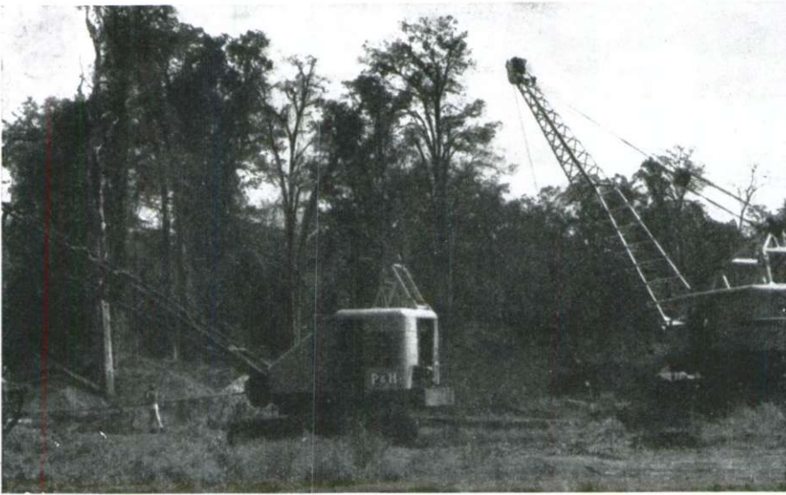
Fig. 13. Mechanization project Shanka. Two draglines of the Dragline-dredging operation. Adola district
