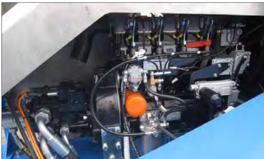
Figure 7. PM50 pump mounted on the engine
