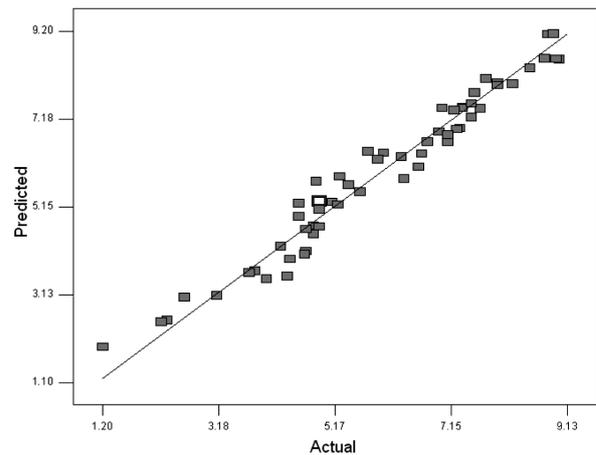
Figure 5: Scatter plot for the weld-nugget size
