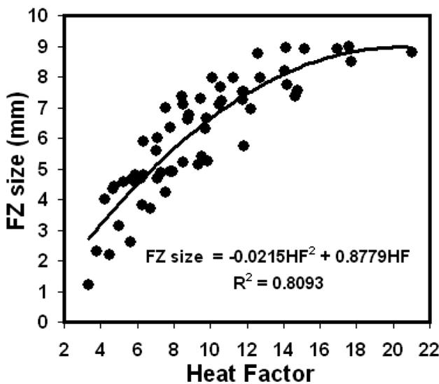
Figure 4: Weld-nugget size versus heat factor (HF)
