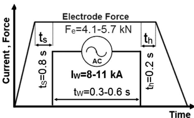
**Figure 1:** Schematic of the welding schedules used in this study
