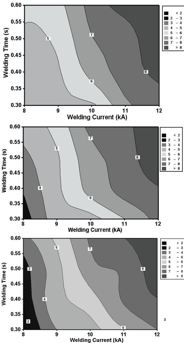
Figure 3: Weld-nugget size versus welding time and welding current at electrode forces of: a) 4.1 kN, b) 5.1 kN and c) 5.7 kN
