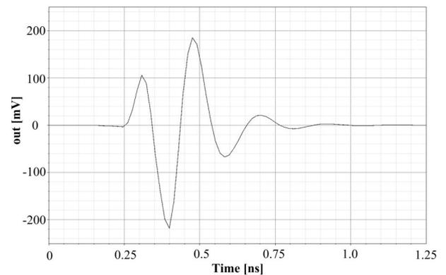
**Figure 3:** Pulse generator output waveform.
