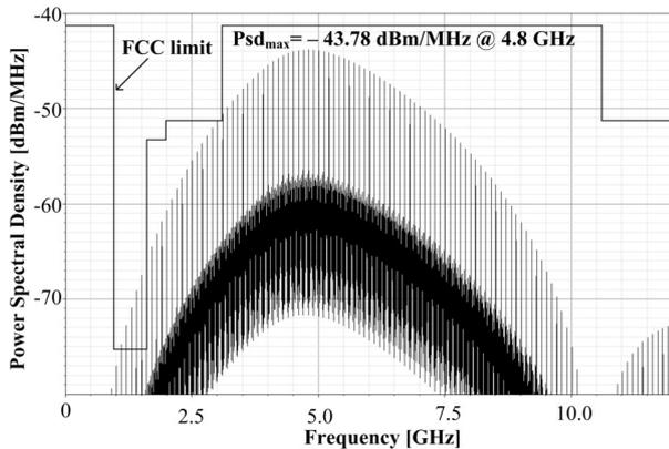
**Figure 4:** Pulse generator output power spectral density.
