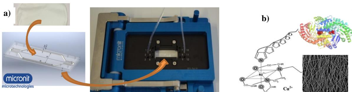
Figure 1: a) Assembly of a resealable flow cell microreactor with nanofiber mat, and b) immobilization principle.
