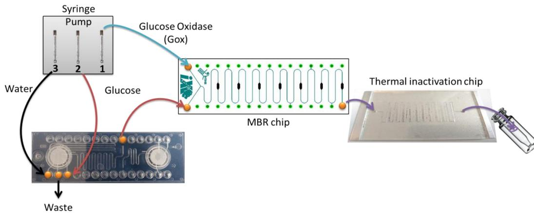
Figure 1: Schematics of “plug and play” assembly of the three microfluidic systems used.
