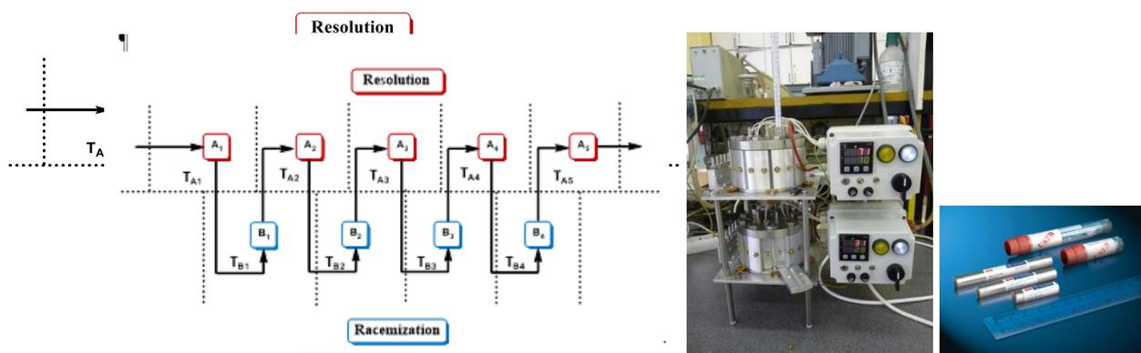
Figure 1: Alternating cascade of reactors for continuous-flow dynamic kinetic resolutions.<sup>2</sup>
