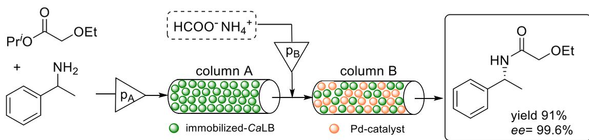
Figure 2: Continuous-flow chemoenzymatic dynamic kinetic resolution of 1-phenylethylamine.<sup>3</sup>
