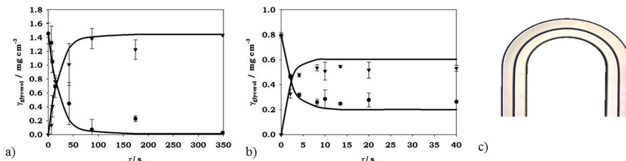
Figure 1: Influence of the residence time on the extraction of glycerol from the biodiesel using a) DES and b) water and c) flow profile for DES:biodiesel system observed under the microscope (— mathematical model)
