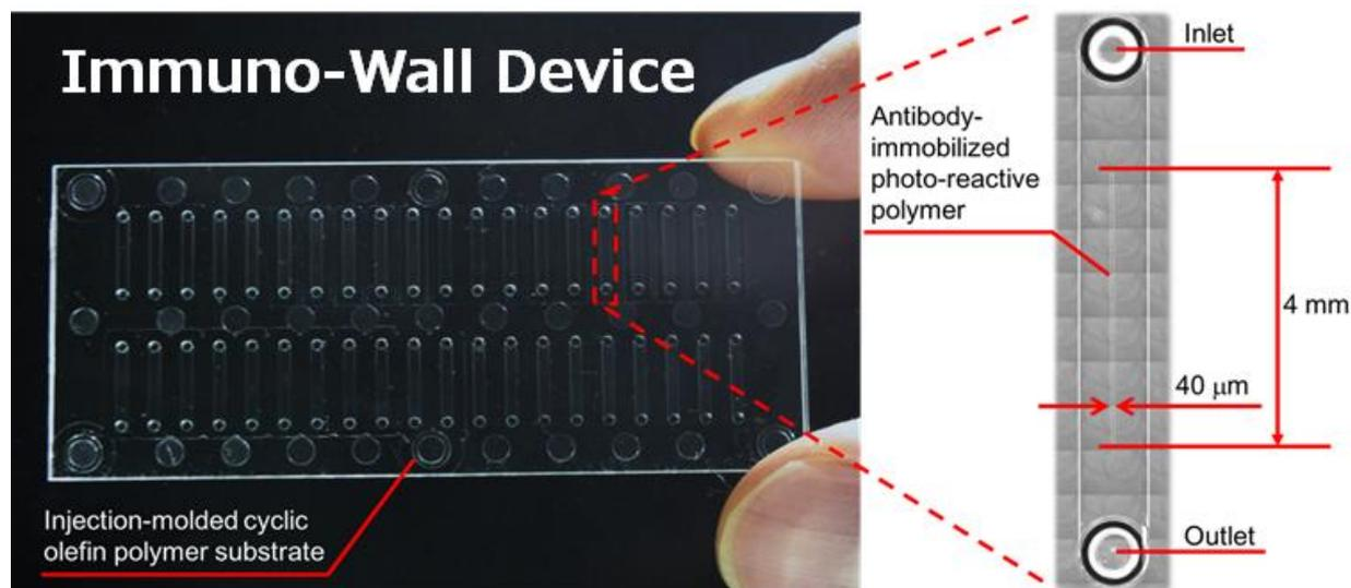
Figure 1: Photo and design of the immuno-wall device (adapted from reference 9)
