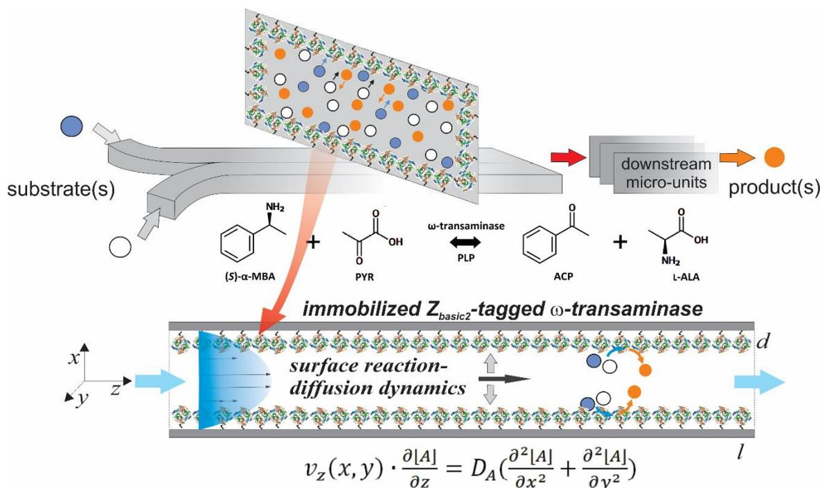
Figure 1: Schematic presentation of the microreactor system with surface-immobilized ω-transaminase.<sup>5</sup>
