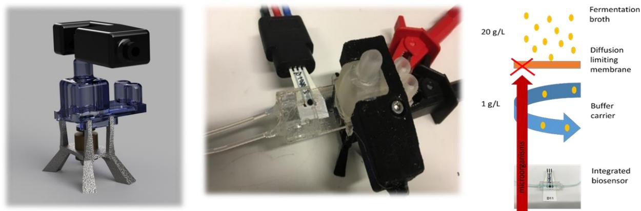
Figure 1: Left: A picture of the micro-bioreactor with integrated OD optical sensor and stand; center: A 3D-printed micro-bioreactor with integrated glucose biosensor and OD optical sensor. -right: Diffusion membrane and sensor scheme.
