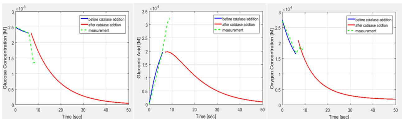
Figure 2: Comparison of concentration profiles for glucose, gluconic acid and oxygen in MBR: simulation results (solid line) vs. experimental data (dashed line).
