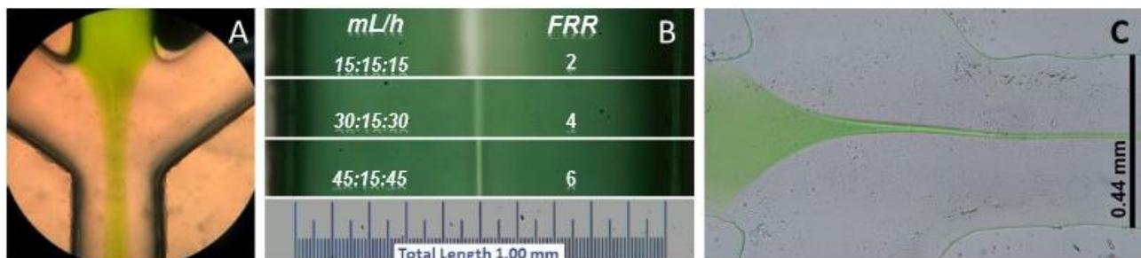
Figure 2: A) Flow focusing in the junction of the 1 mm device used for the synthesis of inorganic colloids (center channel: green dye, side channels: water). B) Different diffusions regimes of water (center channel) and green dye (side channels), for several flow rates in the 1 mm device. C) Flow focusing was also achieved for the junction of the designed 0.1x0.1 mm device, for biological synthesis (center channel: green dye, side channels: water).
