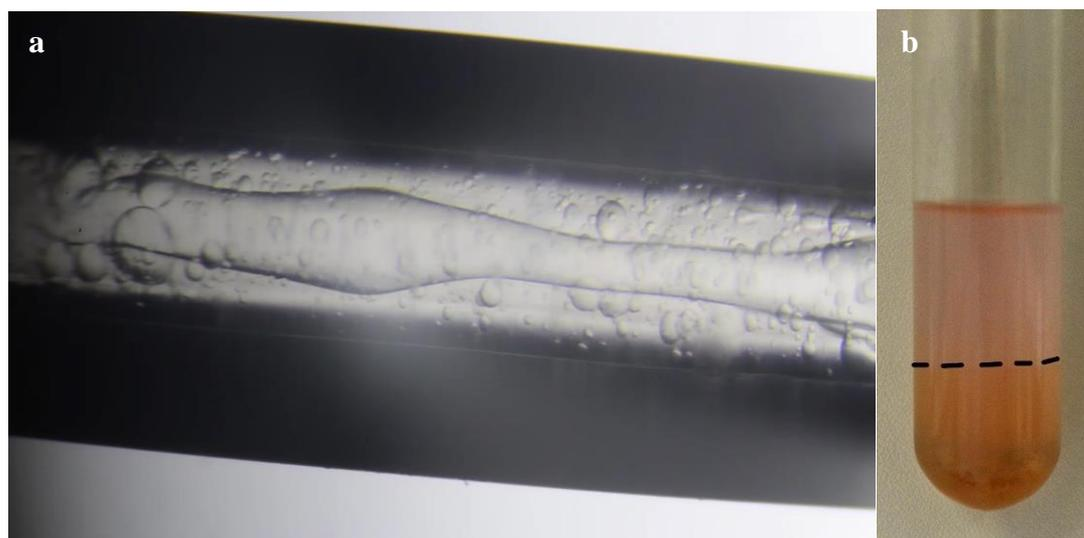
Figure 1: a) Phase separation after less than 1 min residence time within the microchannel; b) AMTP phases at the outlet of the microflow system with characteristic color of R- phycoerythrin in the top phase
