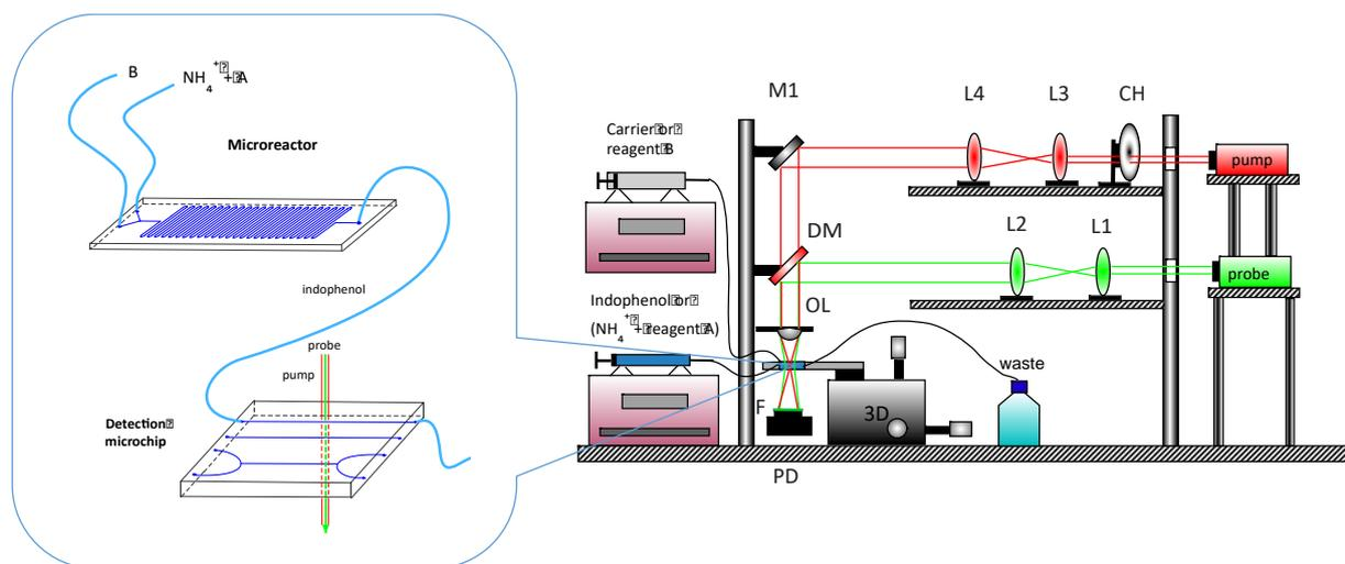
Figure 1.  $\mu$ FIA-TLM system and microchip connection for reaction and detection of indophenol blue.
