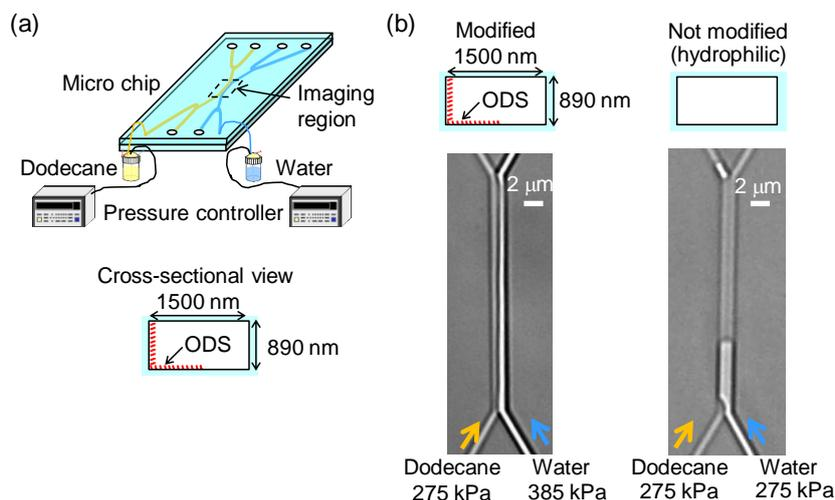
Figure 2: Verification of formation of parallel two-phase flow in nanochannel. (a) Schematic of experimental apparatus. (b) Microscopic image of parallel two-phase flow in 800 nm channel.
