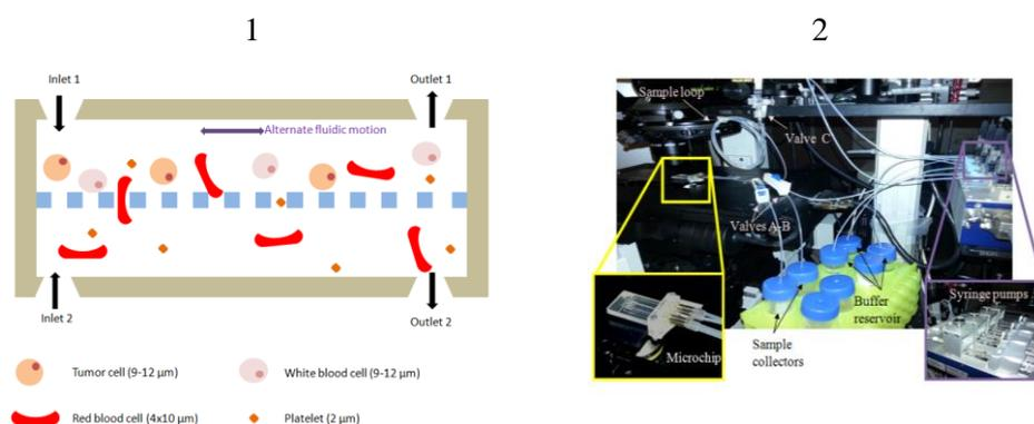
Figure 1: Working principle of the filtering membrane (blue): sample is injected from Inlet 1. Outlet 1 recovers the non-filtered cells; Outlet 2 recovers filtered cells. Inlet 2 is used to inject buffer; Figure 2: Experimental set-up of the microfluidic device
