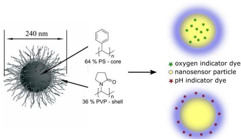
Figure 1: Scheme of PSPVP NPs for oxygen and pH sensing.
