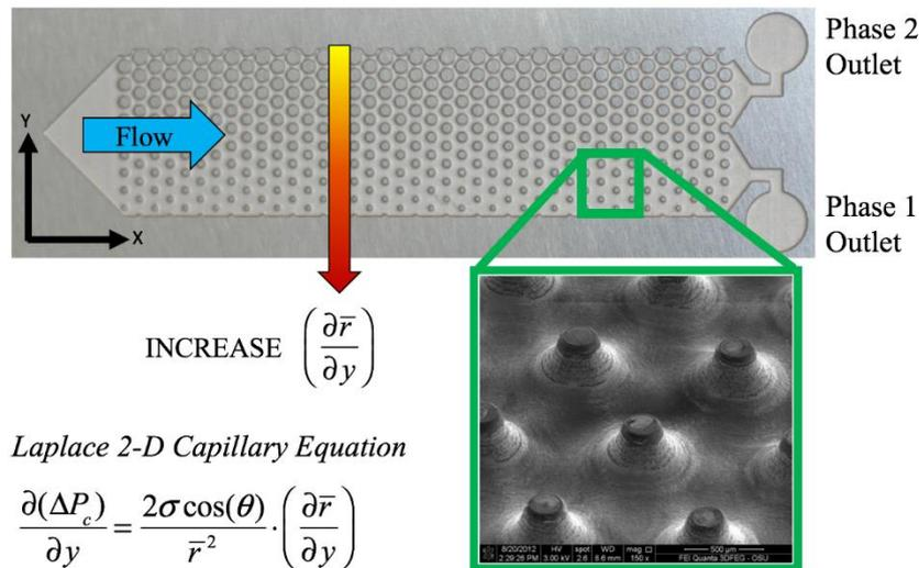
**Figure 1:** Microscale-based flow system with “micropost” features creating a capillary force gradient.
