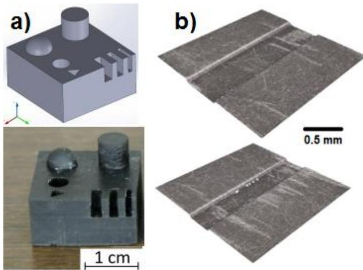
Figure 2. a) 3D model of a test specimen and a printed part. b) 3D scan of low aspect ratio printed microchannels with nominal width 0.6 mm (above) and 0.4 mm (below).
