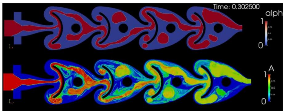
Figure 1: Advanced-Flow™ Reactor CFD simulation results: alph presents aqueous phase/*n*-heptane ratio (aqueous phase is blue, while *n*-heptane is red) and A is normalized concentration profile of MBA.
