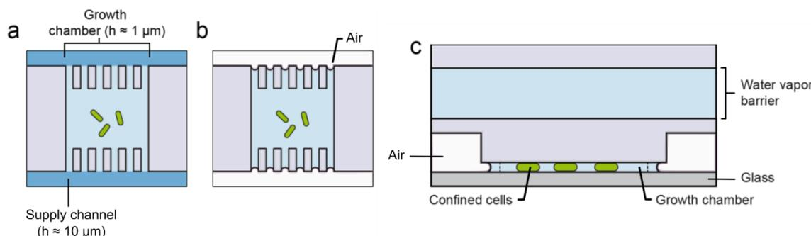
Figure 1: Microfluidic batch cultivation in air-isolated picoliter sized growth chambers: (a) cell inoculation, (b) chamber isolation by the infusion of air into the supply channels, and (c) cross-section of the isolated growth chambers.
