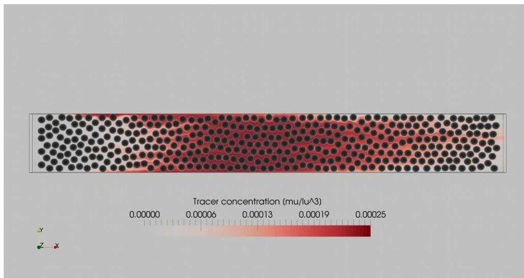
Figure 2: A snapshot of the LBM simulation of the pulse test.
