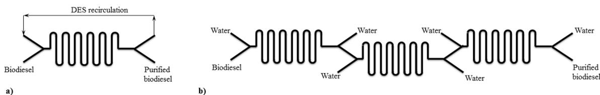
Figure 2: Scheme of proposed microseparation system for glycerol removal using a) DES and b) water
