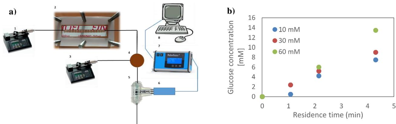
Figure 1: a) Experimental setup scheme and b) glucose concentration at the outlet of the microreactor packed with LentiKats<sup>®</sup> at various flow rates yielding different residence times and with various inlet lactose concentrations stated in the legend.
