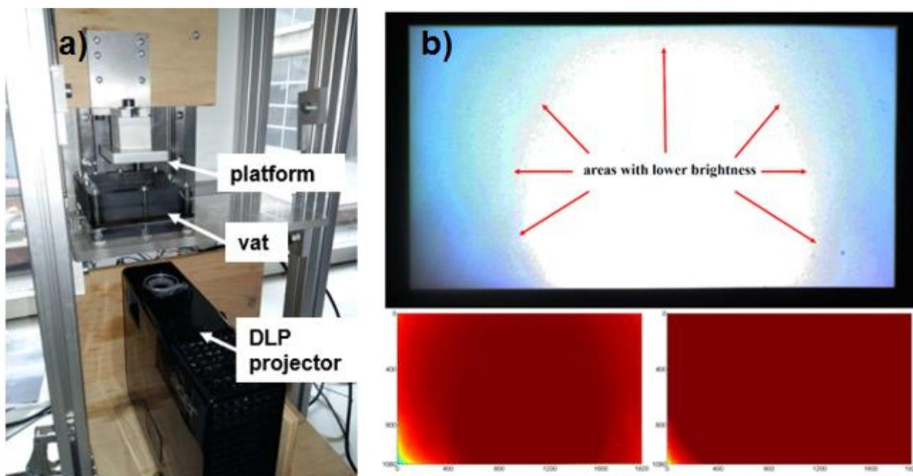
Figure 1. a) Custom made DLP SLA printer with illumination from the bottom arrangement. b) Captured image of the DLP projector illumination. Below: (left) image without mask and (right) image with applied mask. Dark red color represents pixel intensity level of 255.
