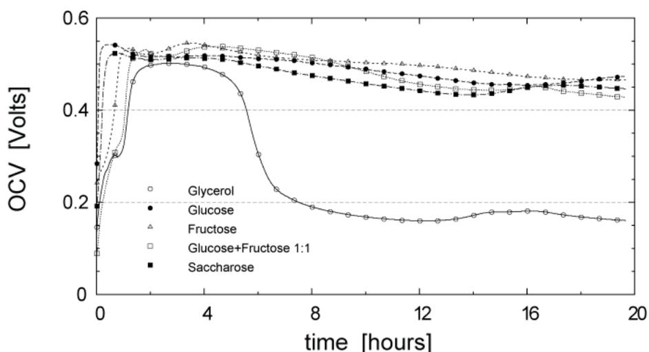
Figure 1: Open cell voltages (OCV) achieved in the yeast cells MFC with various substrates as functions of time of MFC operation.
