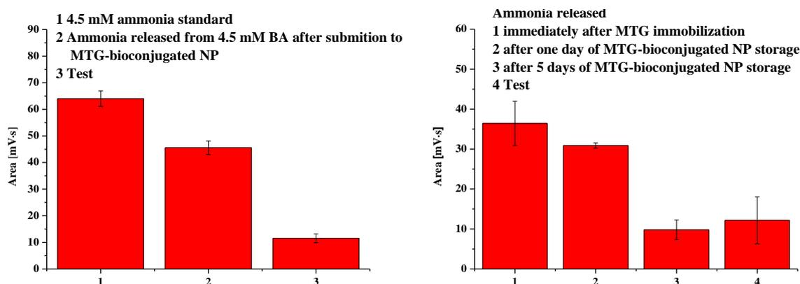
Figure 2. TLM determination of ammonia released from BAs as a result of immobilized MTG activity.
