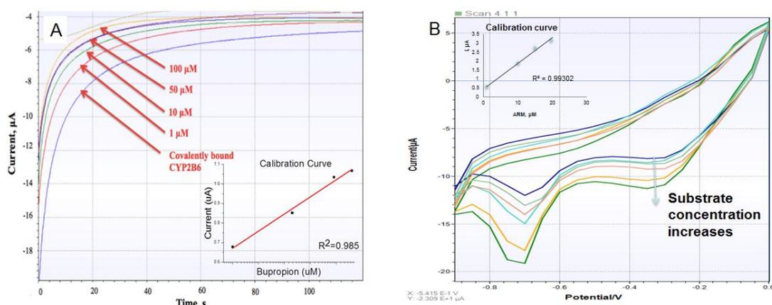
Figure 3: (A) Amperometric response of P450 biosensor to different concentrations of substrate, bupropion. Inset: Obtained calibration curve for the model drug. (B) Cyclic Voltammetry response of P450 biosensor to different concentrations of substrate, artemether. Inset: Obtained calibration curve for the model drug.
