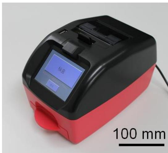
Figure 2: Portable measurement system for the immuno-wall device
