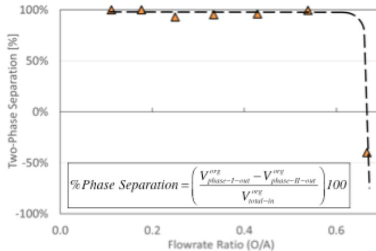
**Figure 3:** Phase separation efficiency as a function of the inlet volumetric flowrate ratio (Organic/Aqueous)
