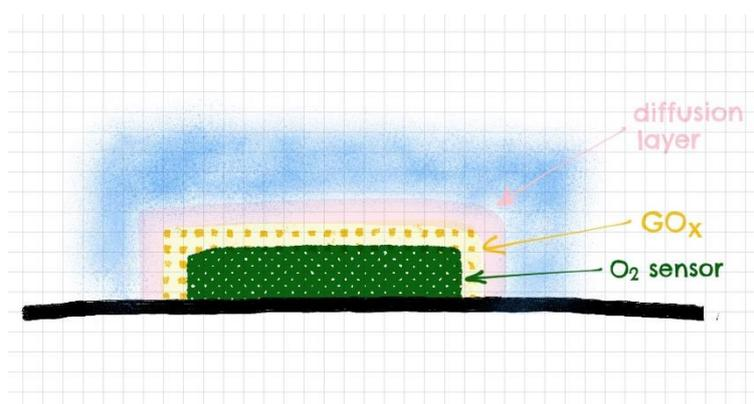
Figure 1: Scheme of glucose sensor employing optical oxygen transducer.
