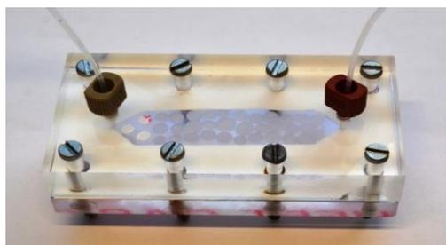
Figure 2: A hexagonal packed bed microreactor with LentiKats<sup>®</sup>.
