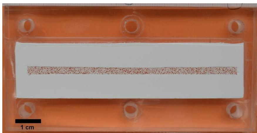
Figure 1: MPBR of dimensions 81.00 mm × 2.94 mm × 0.40 mm, randomly packed with Novozym<sup>®</sup> 435 beads.
