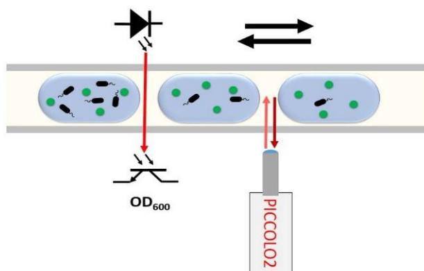
Figure 2: Scheme of on-line, real-time oxygen concentration, pH and OD measurements on microdroplets.
