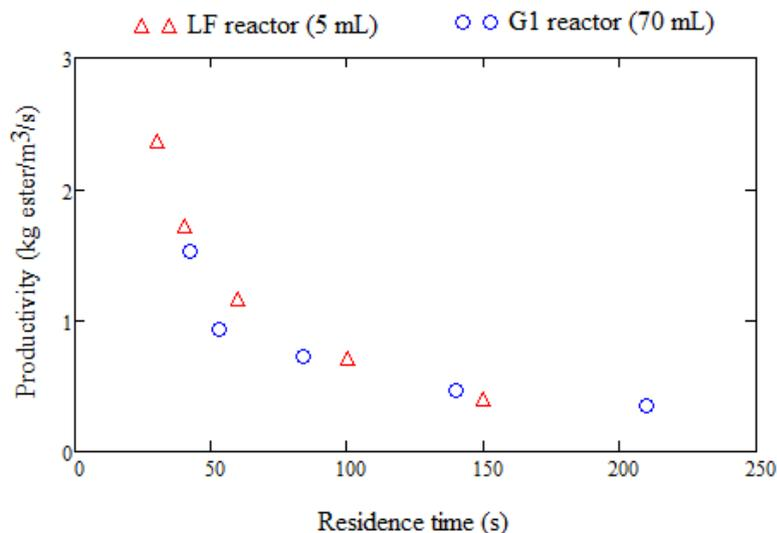
Figure 1: Comparison of the obtained productivity in LF and G1 reactor. Inlet concentrations: CaLB 0.24 g/L, 2 M acetic anhydride and 4 M of isoamyl alcohol in *n*-heptane; flow rate ratio of aqueous phase (0.1 M potassium phosphate buffer with pH 8) and *n*-heptane: 15:85 (% vol.); 30°C
