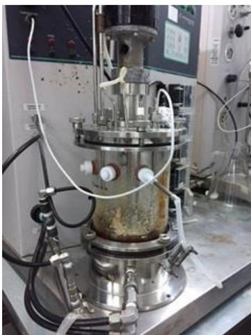
Figure 2: One-liter bioreactor used for the synthesis of biodiesel from waste chicken oil with sol-gel entrapped LipT<sub>6M</sub>.
