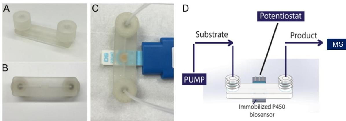
Figure 1: A, B) Photographs of 3D-printed P450 chip, isometric and bottom view. C) Assembled P450 chip with gold electrode biosensor connected to a PalmSens3 potentiostat for online measurements; D) Schematic representation of the P450 chip with a novel biosensor for the online detection of drug-enzyme interactions.
