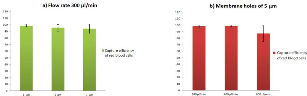
Figure 4: Graphs showing different sorting capabilities with respect to membrane hole dimensions and flow rate – a) Capture efficiency of red blood cells at fixed flow rate and different microdevices; b) Capture efficiency of single microdevice with different mixing flow rate;
