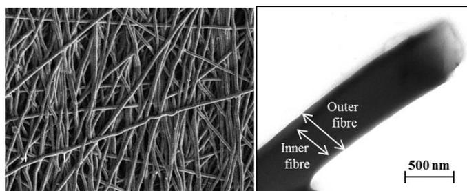
Figure 1. TEM pictures of the coaxial nanofibre membrane.
