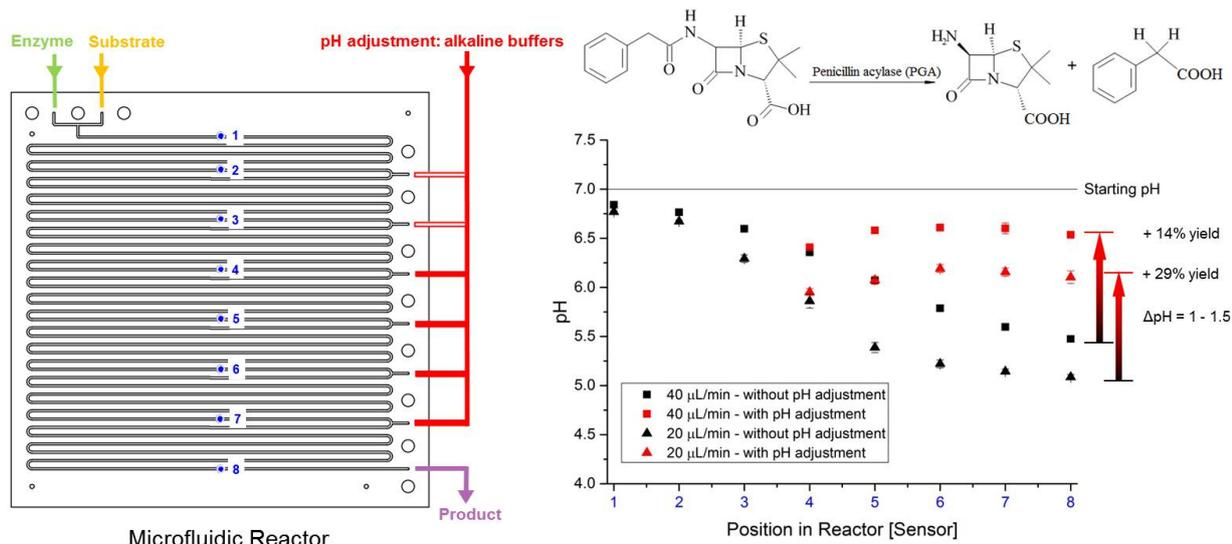
Figure 1: Microfluidic side-entry reactor schematic showing the readout positions of eight sensor spots, one after each side entry (left). pH adjustment of a penicillin G acylase reaction at two different flow rates showing that the stabilization of the pH in the ideal operating range of the enzyme leads to an increase in product yield (right).
