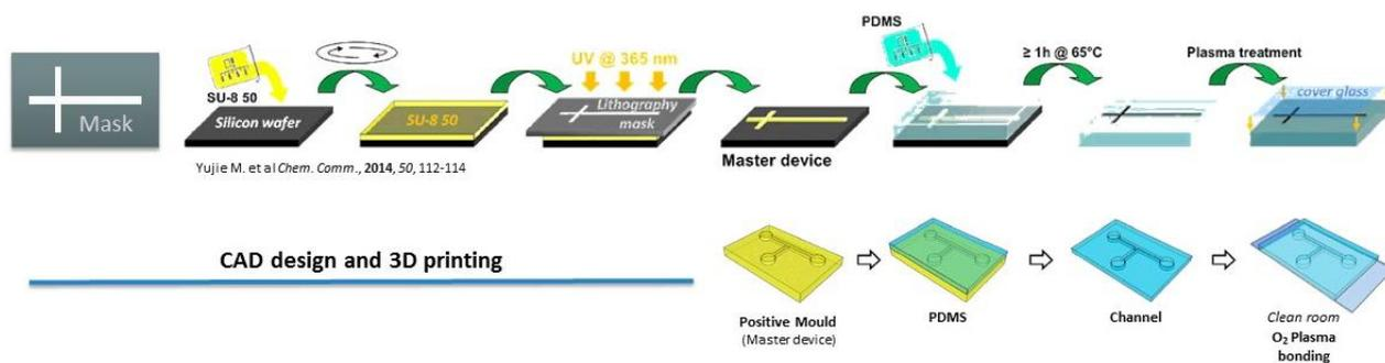
Figure 1: Stepping down the photolithographic process by 3D printing replica mould (3DP-REM).
