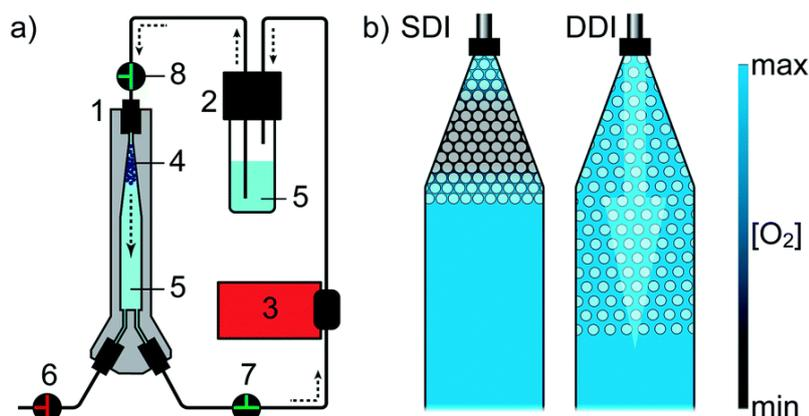
Figure 3: Scheme of 3D printed incubator for cultivation of cells in pL droplets.
