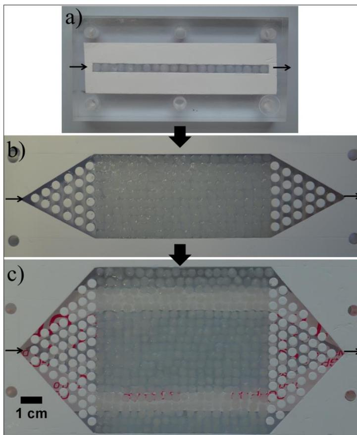
Figure 1: MPBRs presenting the scale-up in channel width, where length and depth were the same: a) an MPBR with cca. 4 mm wide rectangular channel, b) an MPBR with hexagonal channel (rectangular part is cca. 40 mm wide) with triangular inlet and outlet parts containing pillars, and c) an MPBR with hexagonal channel (rectangular part is cca. 80 mm wide) with triangular inlet and outlet parts containing pillars.<sup>4</sup>
