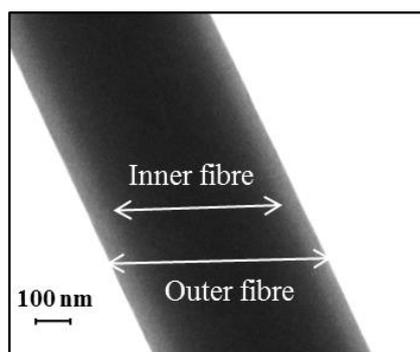
Figure 1: Structure of the coaxial material used for the development of the biosensor. The inner fiber is formed by meso-tetra(pentafluorophenyl)porphine (PtTFPP) solubilized in poly(methyl methacrylate) (PMMA), and the outer fiber is based on PolymBlend<sup>®</sup> (a polymer blend which has been formulated with an optimum mixture of two high molecular weight statistic copolymers to produce materials by electrospinning).<sup>1</sup>
