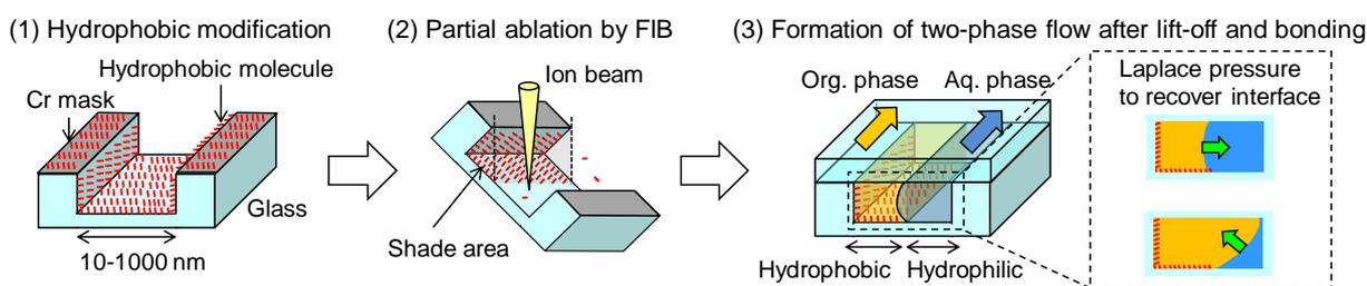
Figure 1: Schematic of partial surface hydrophobic modification method in nanochannel.
