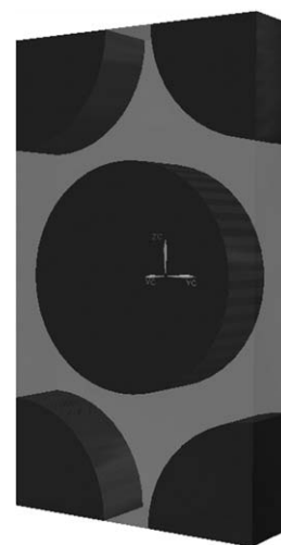
Figure 4: UCE geometry of yarn with V_f = 0.6 (fibers – black, matrix – gray)
