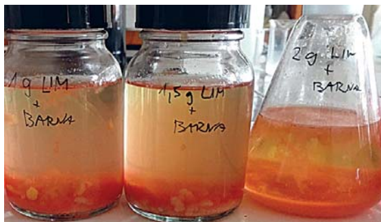
Slika 8: Odpadne vode s pigmentno barvo, čiščene z limoninimi olupki v koncentracijah 5, 7,5 in 10 g/l Figure 8: Pigment printing ink wastewaters treated with lemon peels in concentrations of 5, 7.5 in 10 g/l
