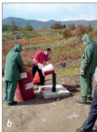
Fig. 8: Places of tracer injections – (a) in the sinkhole near the village Rastovača; (b) in the piezometric well near the village Drežnik Grad.
