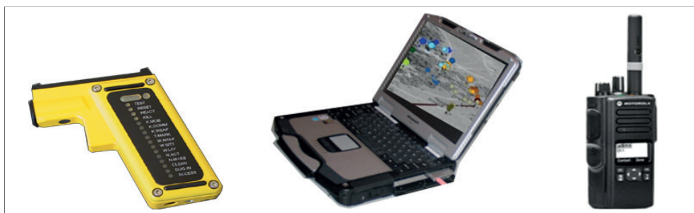
Slika 7: Oprema O/K; Cgun, EXTERM in PRS Motorola DP4601
