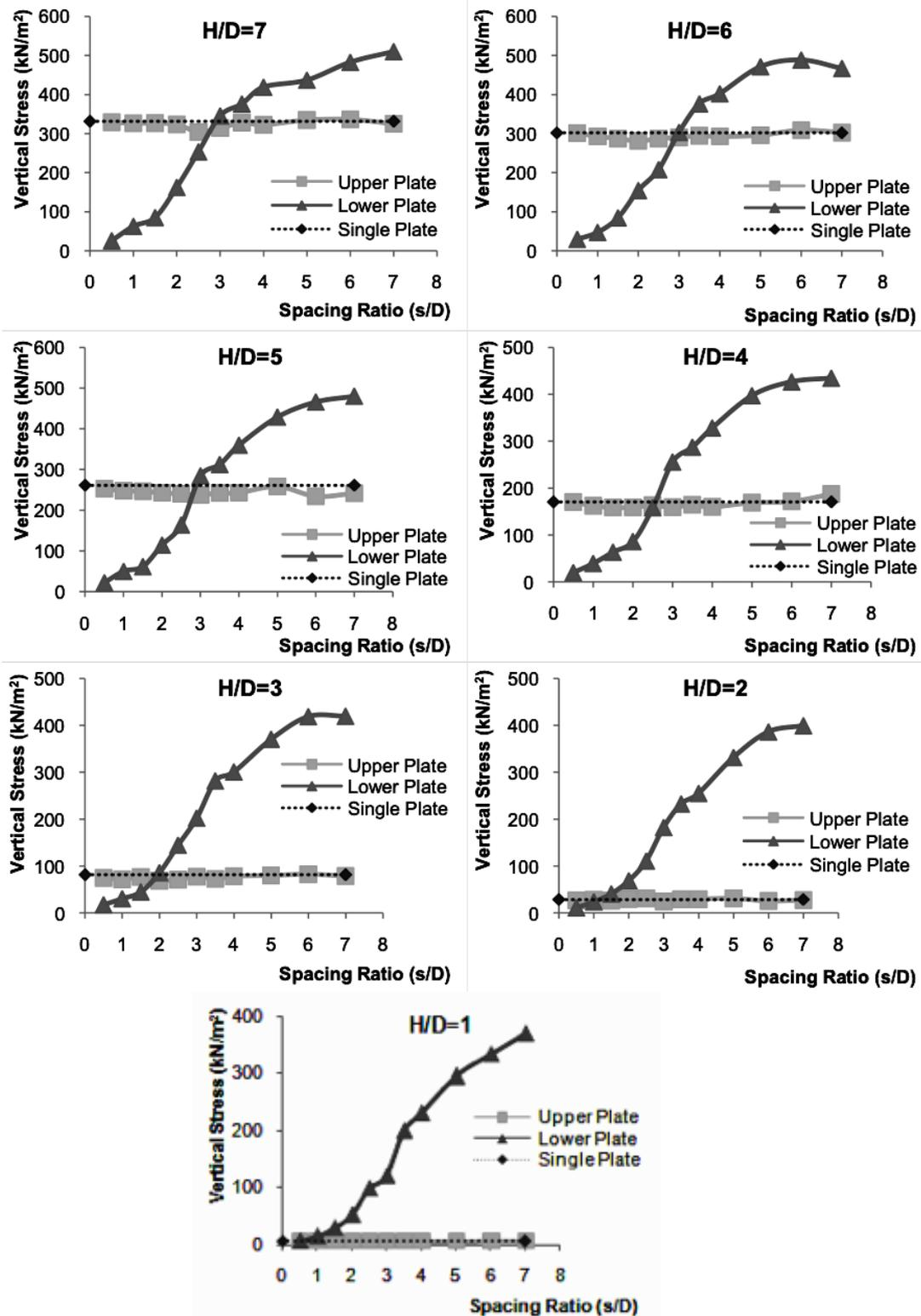
Figure 4. Vertical stress versus spacing ratio for the constant embedment ratios.
