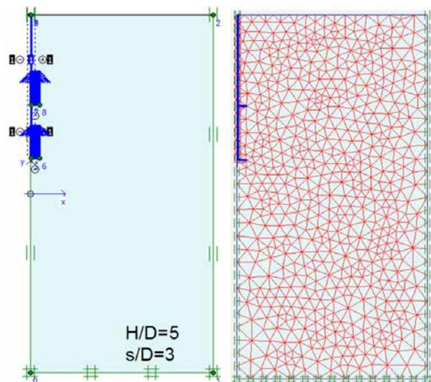
**Figure 2.** Typical finite-element mesh.
