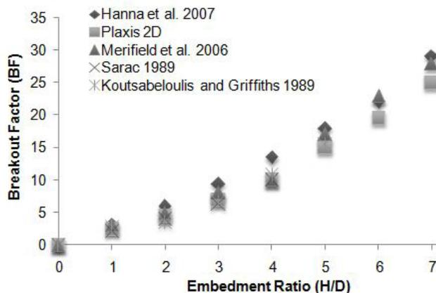
Figure 3. Comparison of the breakout factor for a single plate.
