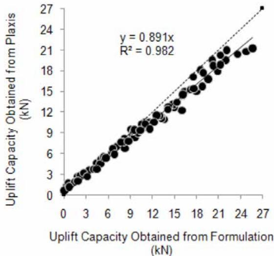
Figure 8. Comparison of the uplift capacities obtained from PLAXIS and formulation (Eq. 4).
