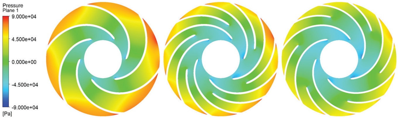
Fig. 9. Pressure distribution in different kinds of impeller
