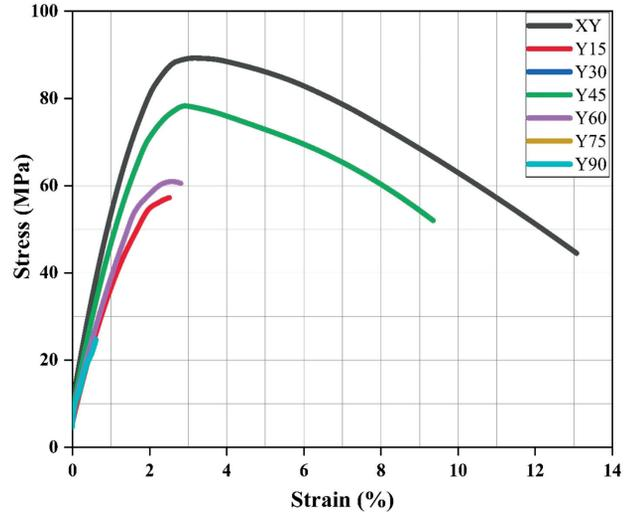
**Figure 7:** Flexural stress-strain graphs for Y-samples
