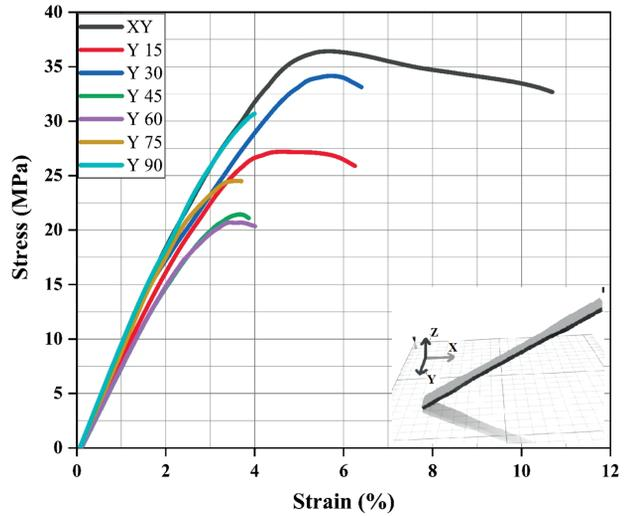
**Figure 4:** Stress-strain graphs for Y-oriented samples
