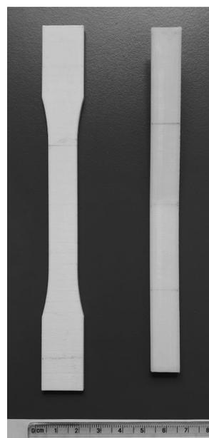
**Figure 2:** Tensile and flexural samples
