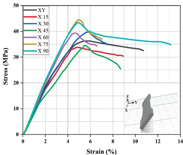
**Figure 3:** Stress-strain graphs for X-oriented samples
