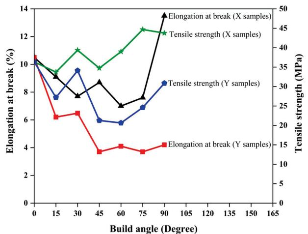
**Figure 5:** Comparison of the failure strain (elongation at break) and tensile strength of the samples printed at different angles to the X- and Y-orientations
