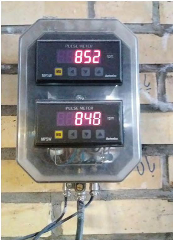
Figure 5: Remote display of yarn feeding speed monitoring system in circular weft knitting machine
