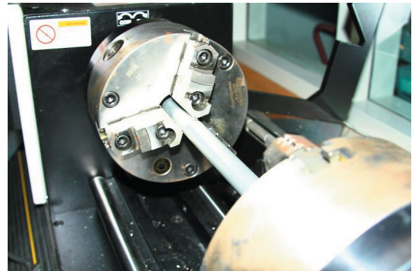
Fig. 6. Mounting of the shaft to the TiniusOlsen torsion testing machine
