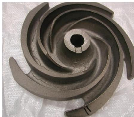
**Slika 4.** Ulita sesalna turbina z žilastimi razpokami**Figure 4.** The casting component "Impeller" with the casting defect veining
