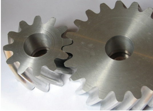
Fig. 17. A pair of the UPT gears; m_n=5\text{ mm} ; z_1=12 , z_2=20
