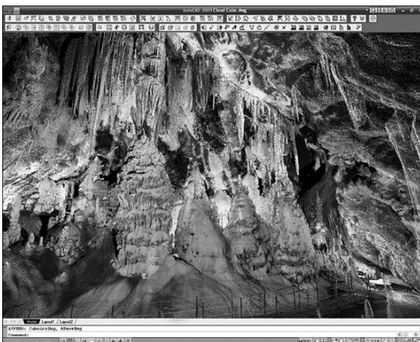
Fig. 7: A detail of the point cloud of Santa Barbara cave visualized on AutoCAD® platform with Virtualgeo’s CloudCUBE software (the location of the visualized detail is highlighted in Fig. 9).
