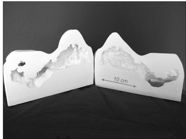
*Fig. 11: The scale plastic model of Santa Barbara cave produced with rapid prototyping 3D printer.*
