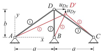
$$L'_1 = \sqrt{(a + u_{Dx})^2 + (b + u_{Dy})^2} = 5.00415 \text{ m},$$
