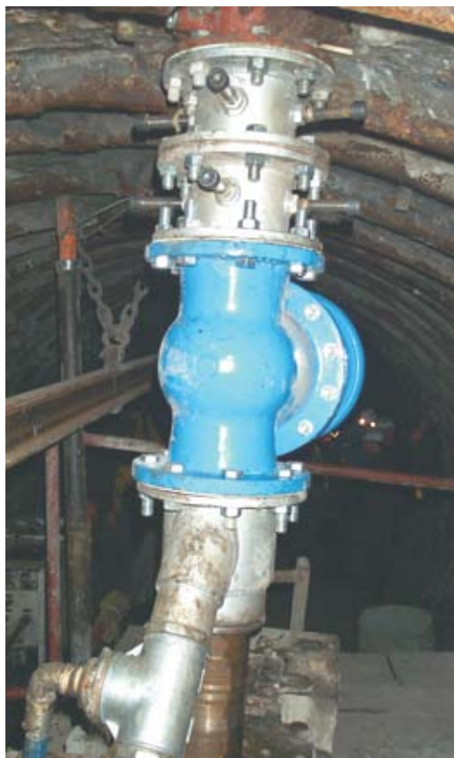
Figure 4. A flange of the conductor pipe, brakes, a valve, and a swivel pipe
