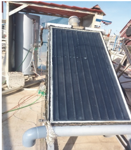
Solar water flat plate collector with air absorber cooling
