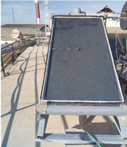
Solar air flat plate solar collector
