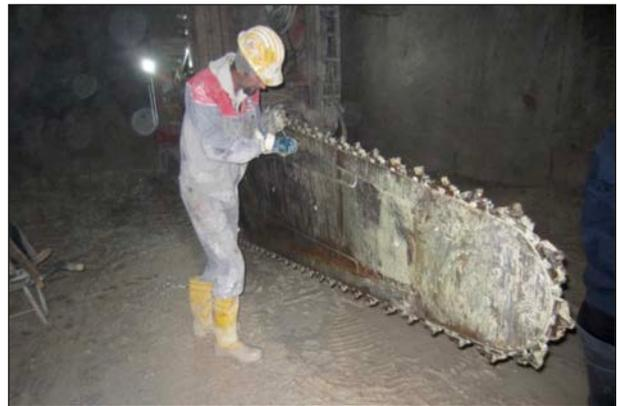
Figure 4. Diamond wire and chain cutting machine.
