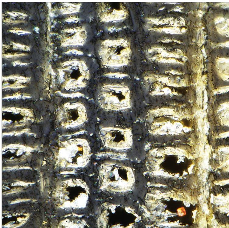
Figure 4. Cell lumina filled with crystals of the fire retardant Burnblock. The image was obtained with confocal scanning laser microscope (field of view  $128 \mu\text{m} \times 128 \mu\text{m}$ ). Colours are not always representative.
