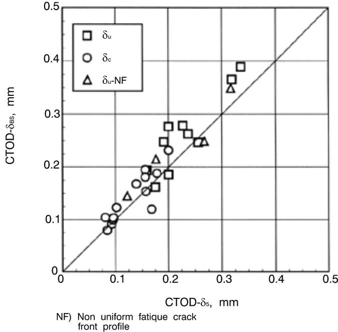
**Figure 2:** Comparison of directly measured ( $\delta_5$ ) and calculated ( $\delta_{BS}$ ) CTOD fracture toughness values of specimens  $B \times 2B$  with a deep crack ( $a/W = 0.5$ ) in homogeneous and heterogeneous under-matched weld joints
