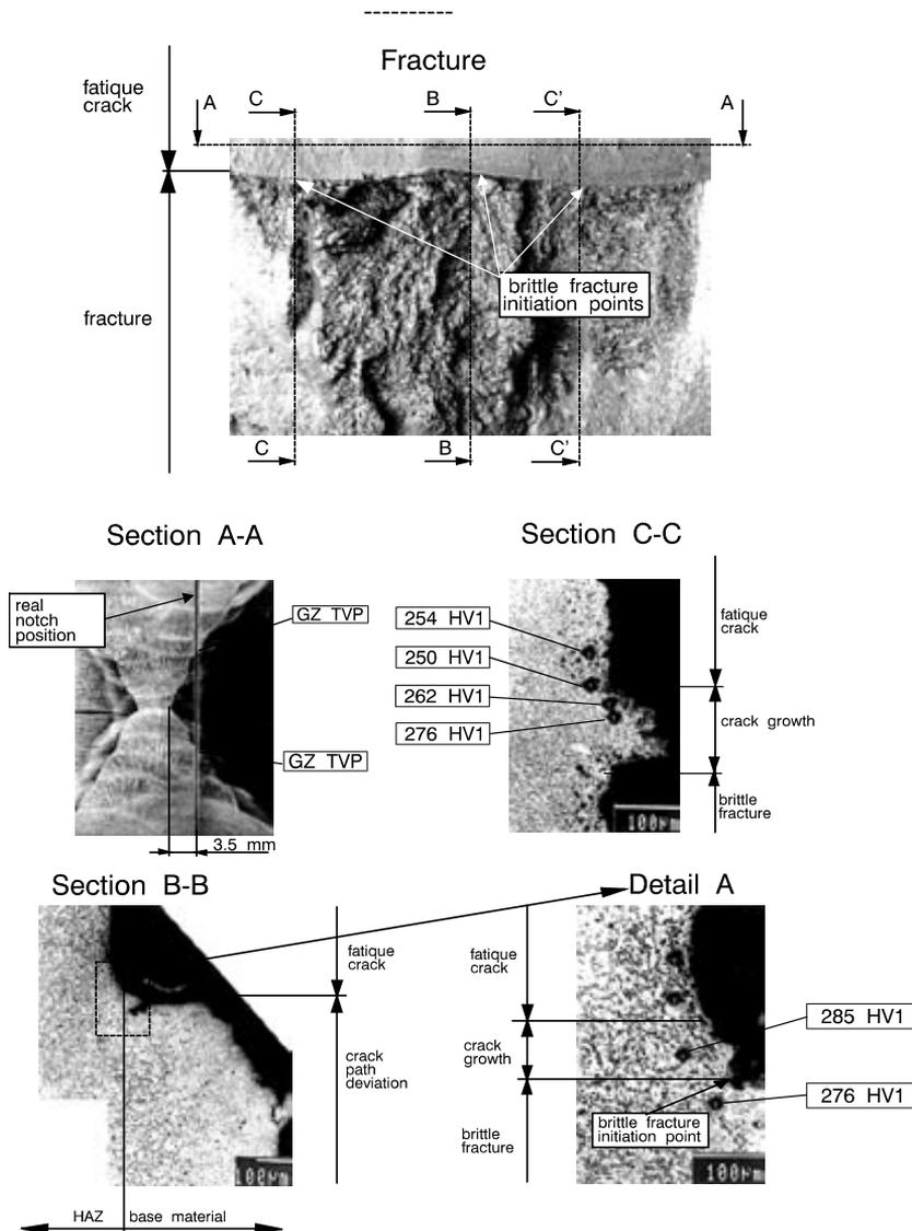
**Figure 1:** Brittle fracture initiation points and crack path deviation on fractured specimen B × 2B with deep crack in HAZ of the heterogeneous under-matched weld joint
