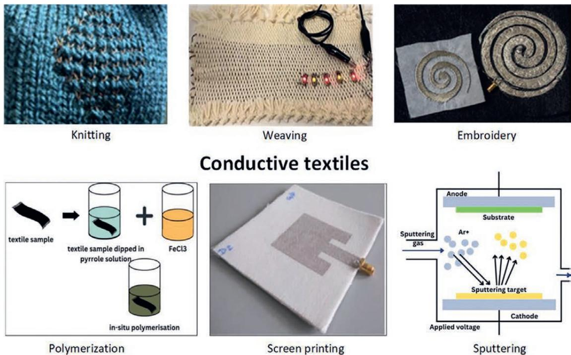
Figure 1: Different manufacturing techniques of conductive textiles:
