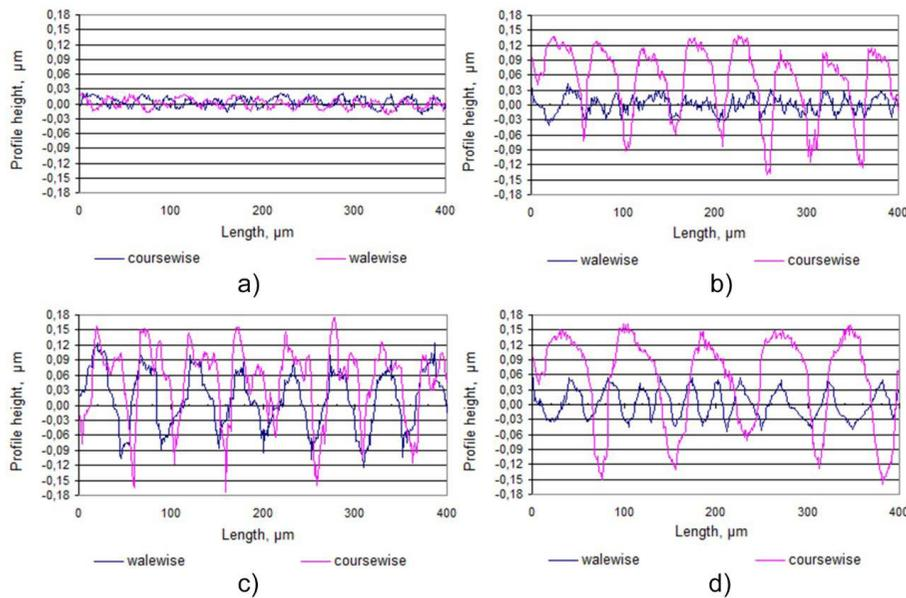
Figure 2: Roughness profiles of cotton knitted fabric samples: a) single plain; b) 1x1 rib 150 g/m<sup>2</sup>; c) French piqué; d) 1x1 rib 280 g/m<sup>2</sup>
