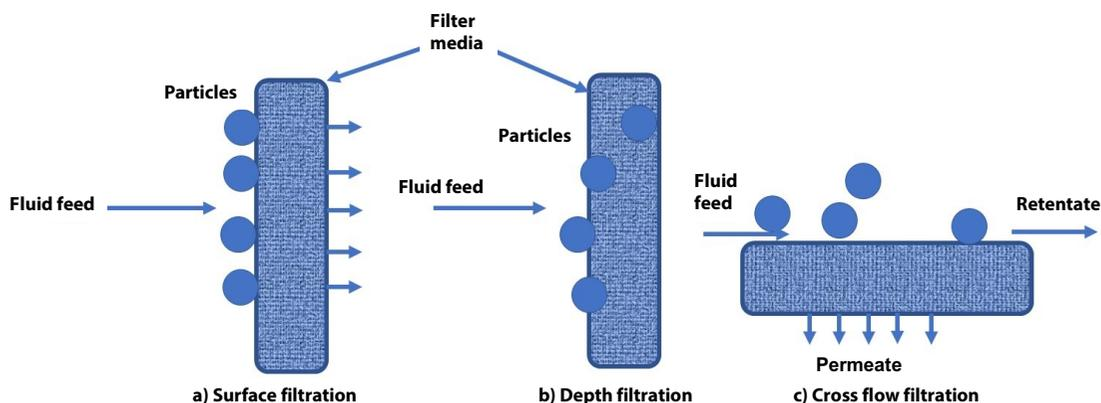
Figure 1: Filtration mechanism [8–13]
