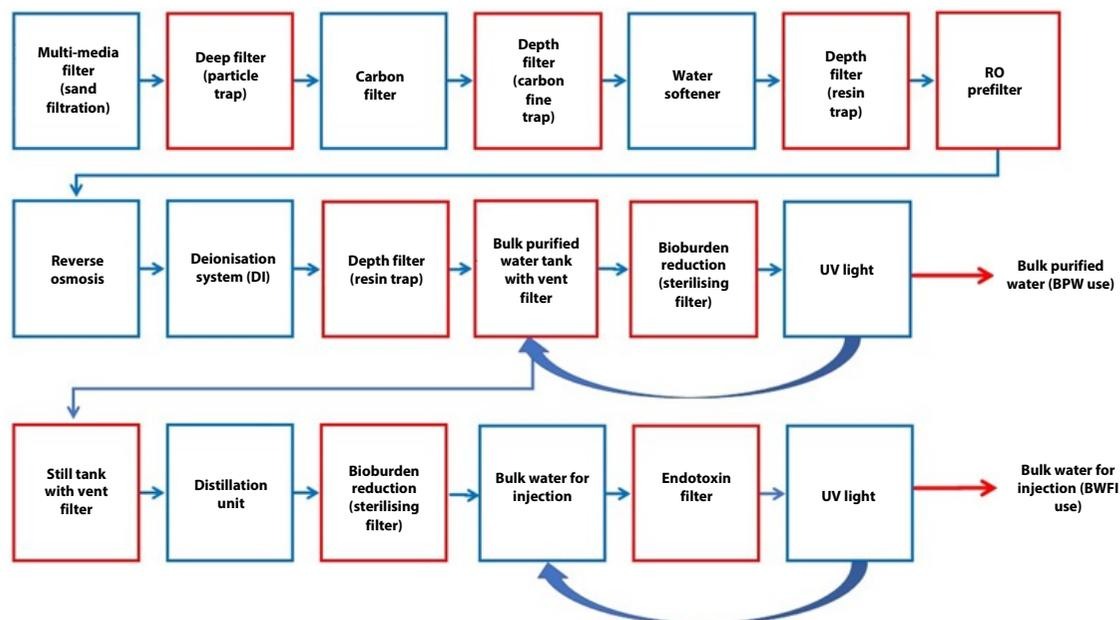
Figure 2: Filtered water system for pharmaceutical use [2, 21, 24, 25, 27, 28]
