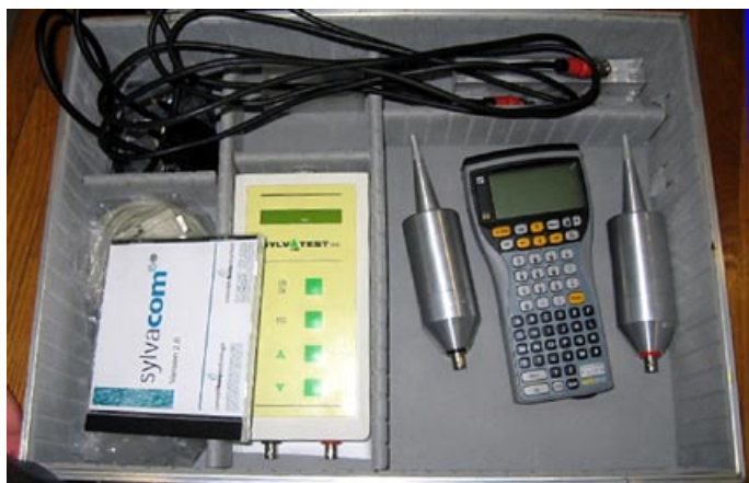
■ Slika 3. Ultrazvočna naprava „Sylvatest Duo“ (merilni inštrument, sondi, računalnik in program Sylvius za obdelavo meritev) Figure 3: Ultrasonic device „Sylvatest Duo“ (measuring instrument, probes, computer and software Sylvius)
