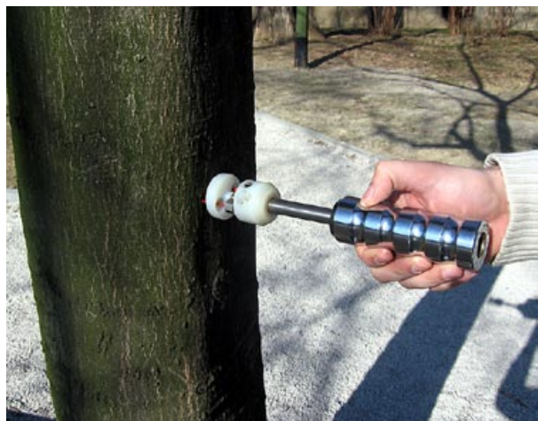
■ Slika 2. Meritev vlažnosti v lesa v naravi Figure 2. Measuring of moisture content of wood in natural environment
