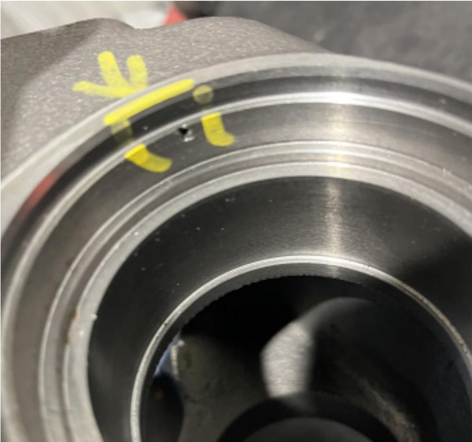
*Figure 7: Visible porosity on machined surface [9]*
