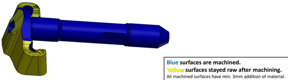
Figure 9: 3D model of a KozolenBoltzen bracket pin sample part [9]
