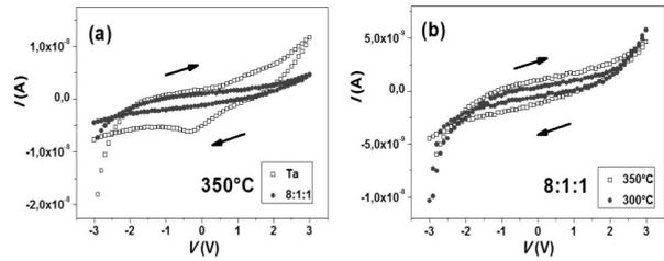
**Figure 4:**  $I-V$  curves of Ta<sub>2</sub>O<sub>5</sub>-based thin films measured with the minimum delay time. The voltage was swept from the negative to positive values and back as indicated by the arrows in the figures.
