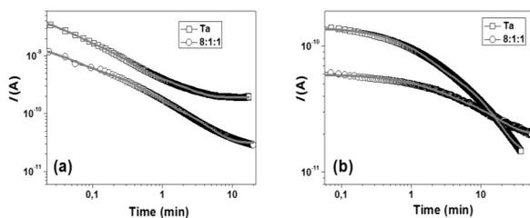
**Figure 5:** Current transients of the Ta and 8:1:1 thin films heated at 400 °C (a) and 250 °C (b), upon applying a constant voltage of 1 V. The solid lines are the fits to the current data with the third- (a) and the second-order (b) exponential decay, respectively.
