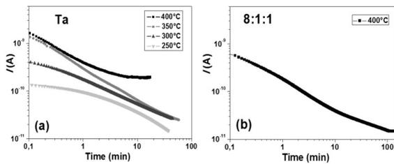
**Figure 3:**  $I-t$  characteristics of the Ta thin films series (a) and the 8:1:1 sample processed at 400 °C (b), measured under the applied voltage of 1V.
