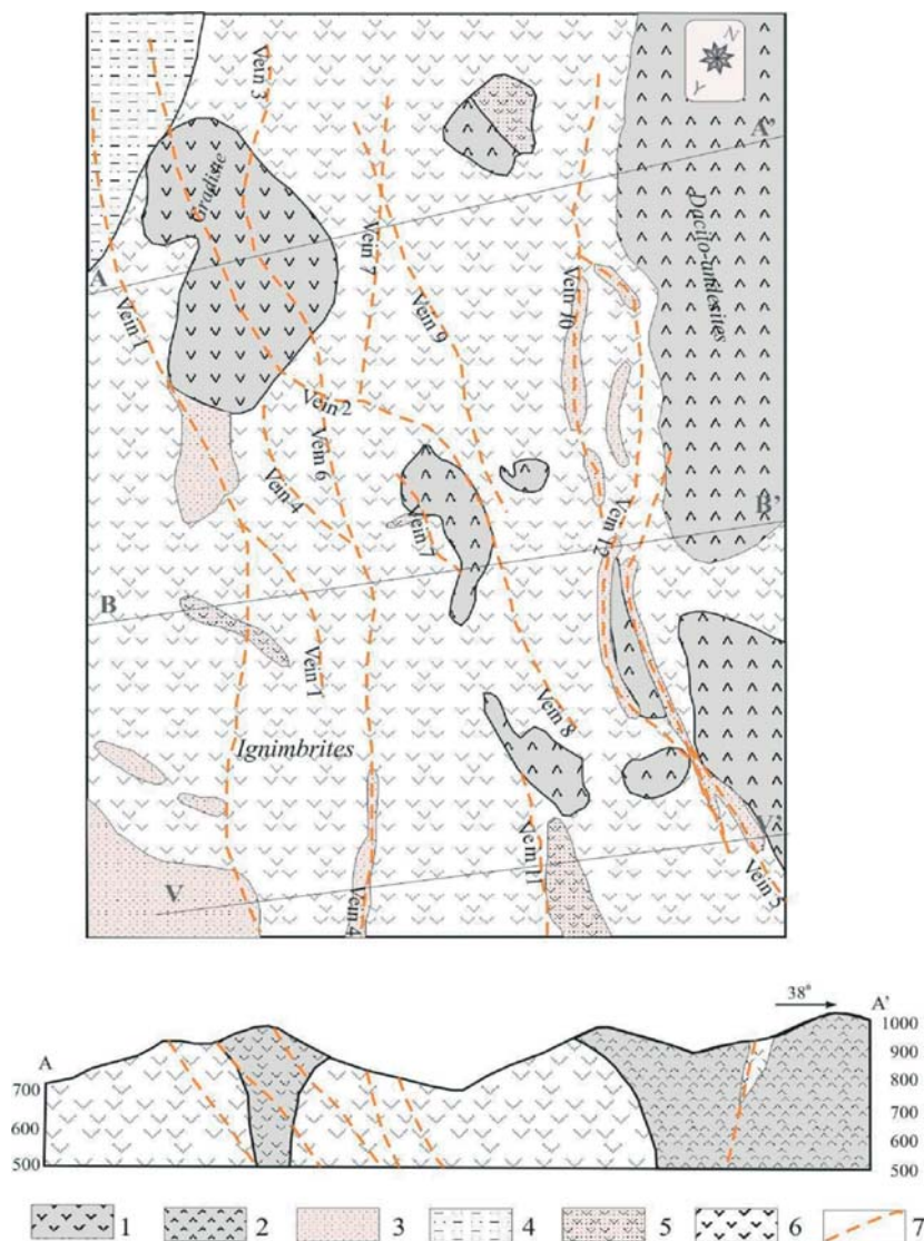
Figure 1. Geological map and cross section of the Pb-Zn Zletovo ore deposit (SERAFIMOVSKI, 1990)
