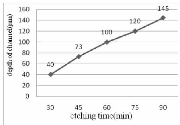
Fig. 1. Depth of channel vs. etching time
