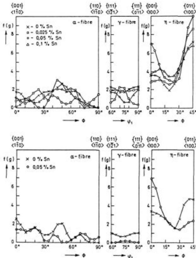
**Figure 4:** Fibre diagram of recrystallized texture for electrical steels measured a) in the middle plane and b) on the surface
