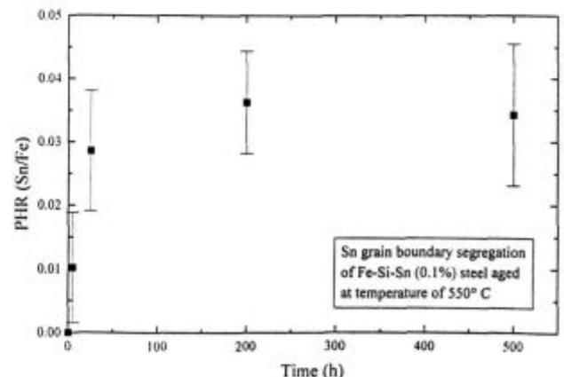
**Figure 1:** Peak height ratio (PHR) between the dominant Sn(M<sub>5</sub>N<sub>45</sub>N<sub>45</sub>) and the Fe(L<sub>3</sub>M<sub>23</sub>M<sub>54</sub>) Auger transitions at the kinetic electron energy of 430 eV and 651, respectively, in dependence of different ageing time
