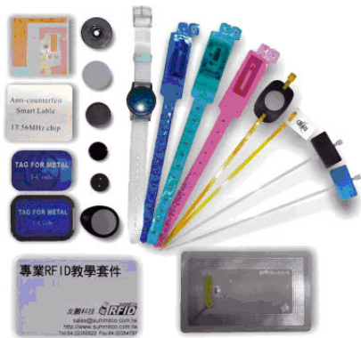
Fig. 1. Various forms of RFID tags (Summit Automation Co., Ltd.)
