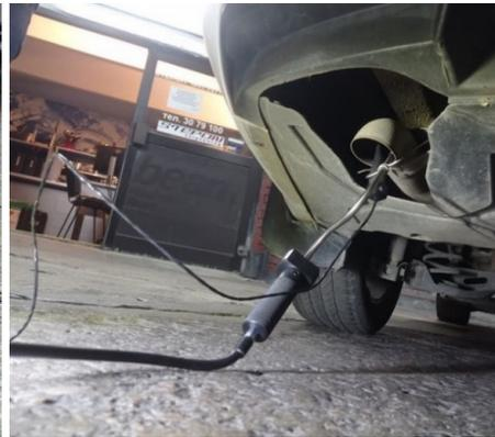
**Figure 5:** Exhaust probe
