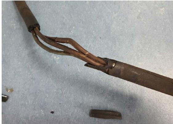
*Figure 5: Part of the degraded cable sample*
