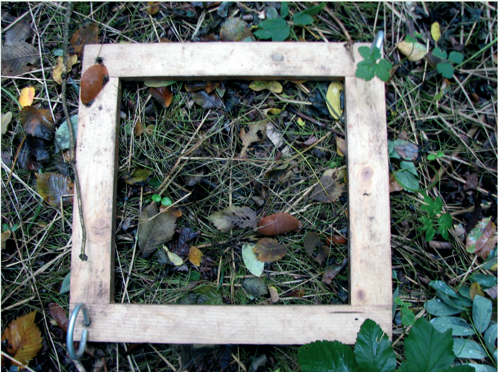
Figure 4: Volume samples of organic sub-horizons were taken using a wooden frame, fixed in the ground by pegs
