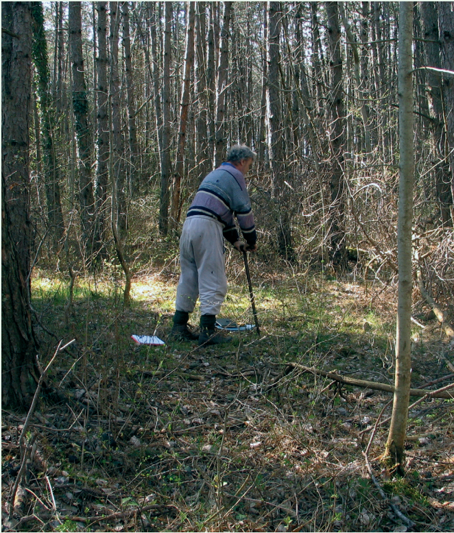
Slika 3: Preiskava talnih razmer s polstožčasto sondo Figure 3: Research of the site condition using a semi-conical probe
