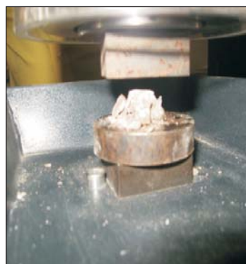
Figure 2. Tests crushing grain by grain.
