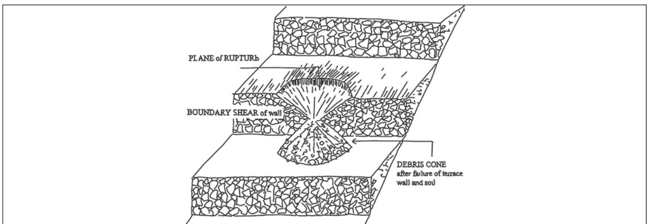
**Figure 12: Schematic view of a collapsed terrace.**
