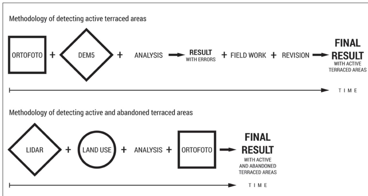
Figure 10: The workflow difference between analysis with and without the detailed LIDAR dataset. The first final result shows only active terraced areas. The second less time-consuming and more precise approach indicates not only active terraces but also abandoned terraced areas.
