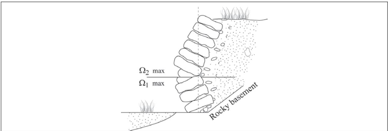
**Figure 8: Wall bulge on the 1/3 lower section.**
