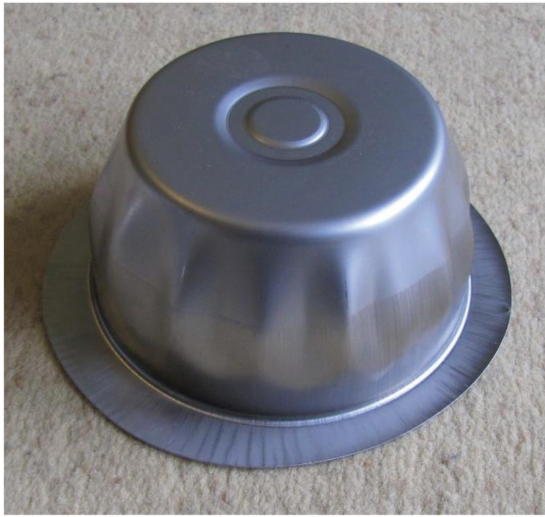
Figure 3: Wrinkling on the conical part of the drawn product.
